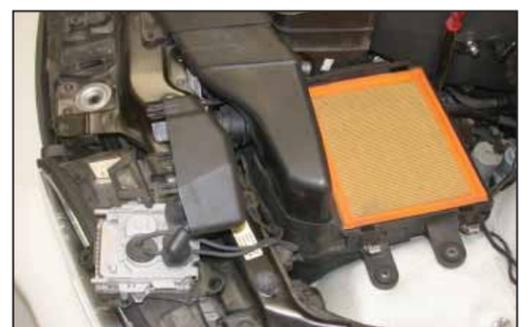
6. Lift the head light module and place out of the way on the core support to gain access to the lower air box for removal.
