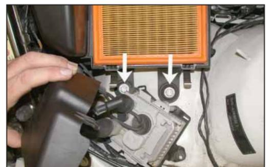
5. Remove the cover to the head light module to gain access to the air box bolts and module nut. Remove the bolts and nut.
