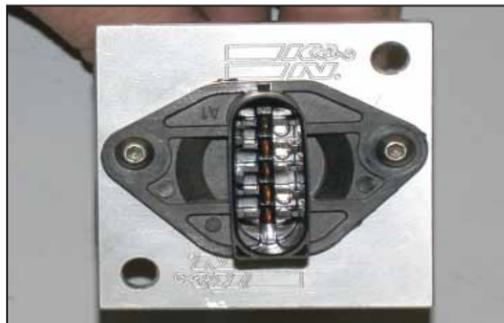
18. Install the mass air sensor into the mass air adapter as shown, secure with the provided hardware.
