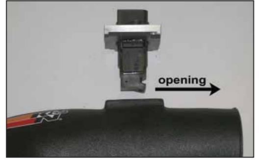
19. Install the mass air sensor assembly into the K&N® intake tube.
