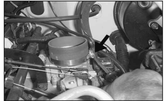
18. Attach the silicone hose to the throttle body using the provided hose clamp.
