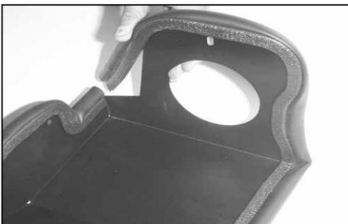
9. Install trim seal onto the heat shield.
