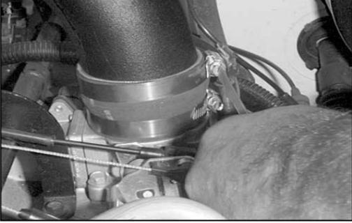
21. Tighten the hose clamp on the silicone hose at the intake tube.
