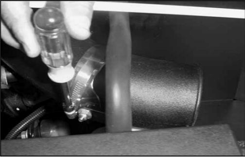
20. Secure the intake tube to the saddle bracket using the provided hose clamp.
