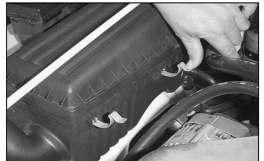
4. Release the 5 over center clips that retain the air box top to the air box base.
