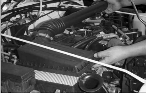
6. Detach the intake tube from the throttle body and remove the entire upper air intake assembly.
