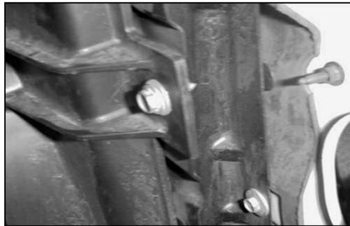
11. Loosen and remove the upper radiator shroud's retaining bolt.
