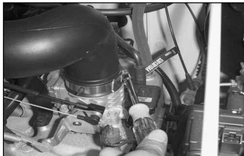
3. Loosen the hose clamp on the intake tube at the throttle body.
