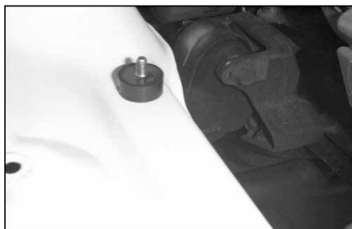
13. Install the second rubber mount stud into the lower air box mounting point using the provided hardware.
