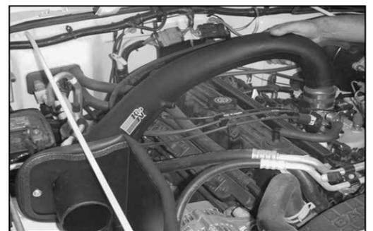
19. Install the K&N® intake tube.
