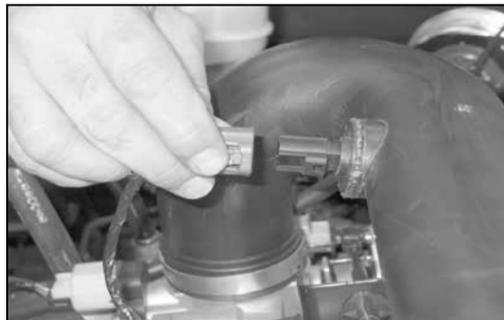
3a. On vehicles equipped with a temperature sensor, depress the temperature sensor electrical connection locking tab and then pull on the connector to disconnect the connection.
