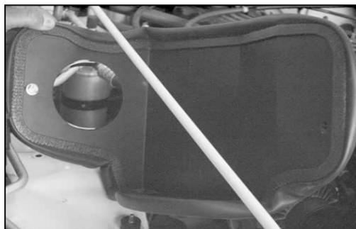
16. Install the heat shield assembly.
