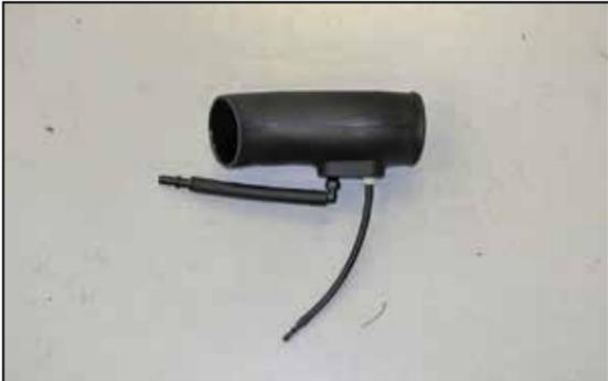
11. Install the vent hose assemblies onto the fittings installed into the K&N® intake tube.
