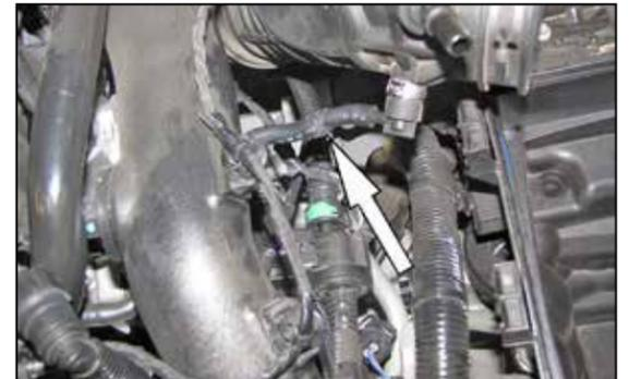
6. Disconnect the solenoid vent hose from the fitting installed into the factory intake tube.
