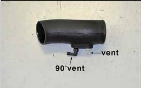
9. Install the provided 1/4npt vent fittings into the K&N® intake tube as show.
