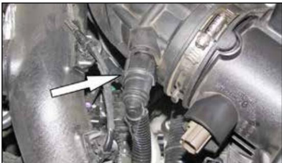
3. Disconnect the crank case vent connection.
