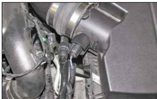
18. Reconnect the inlet air temperature sensor electrical connection.
