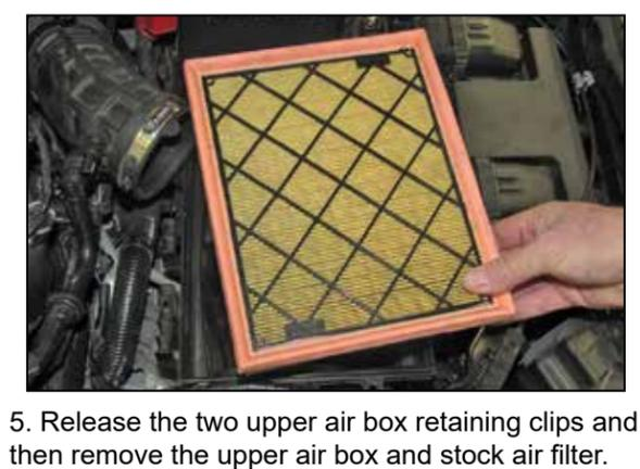
5. Release the two upper air box retaining clips and then remove the upper air box and stock air filter.
