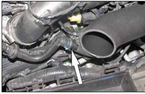
14. Connect the factory crank case vent hose to the quick connect fitting/vent hose installed into the K&N® intake tube.
