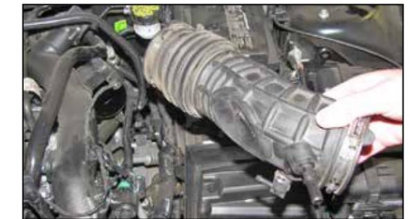
7. Loosen the hose clamp securing the factory intake tube to the turbo inlet and then remove the hose from the vehicle.
