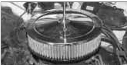
10. Using the provided hardware, secure the air cleaner assembly as shown.
