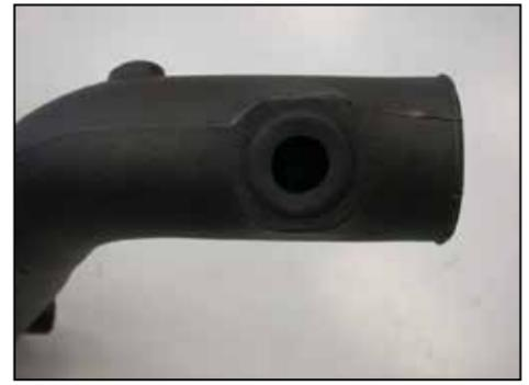
22. Install the supplied grommet into the K&N intake tube as shown.
