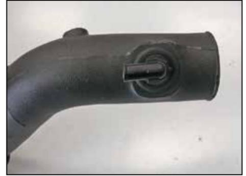
23. Install the stock crankcase vent fitting into the grommet that was installed in the K&N intake tube in the previous step.
