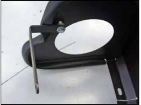
14. Install the "L" bracket onto the heat shield using the supplied spacer between the heat shield and bracket.
