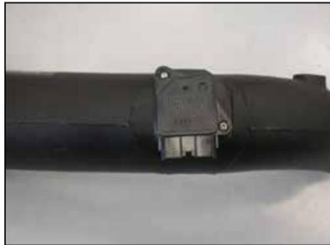
21. Install the mass air sensor assembly into the K&N intake tube using the supplied hardware.
