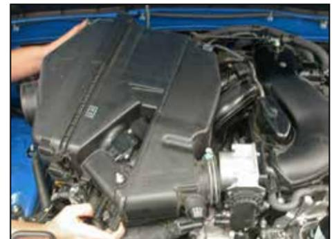
9. Lift up and remove the airbox assembly from the engine.
