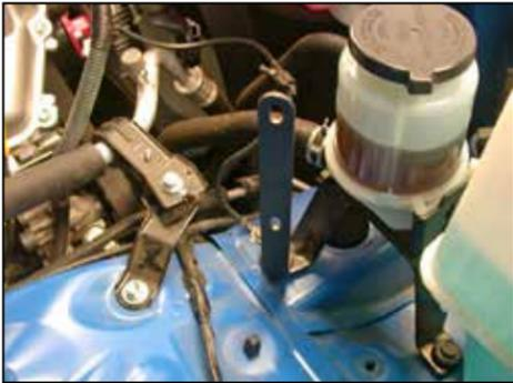
13. Install the "L" bracket onto the power steering reservoir using the bolt removed in step #12.
