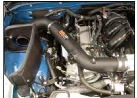
27. Install the K&N intake tube into the silicone hose at the throttle body and align with the saddle clamp. Secure the intake tube with the provided hose clamps.
