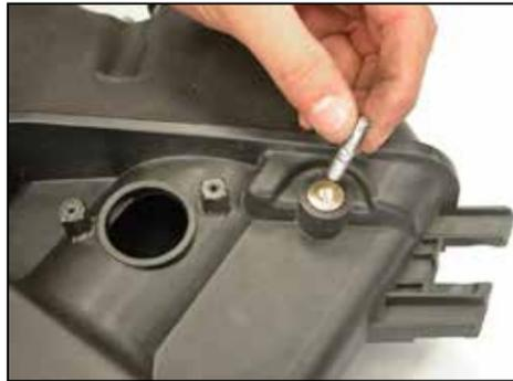
19. Remove the engine cover mounting stud from the airbox as shown.
