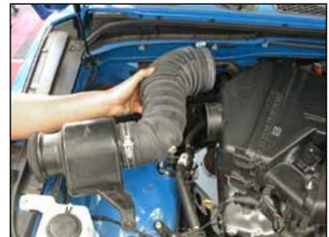
7. Loosen the hose clamp that secures the intake tube to the stock air filter housing, then remove the intake tube and resonator assembly.
