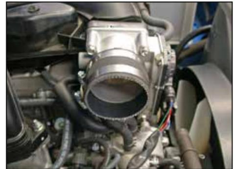
26. Install the silicone hose (08434) onto the throttle body and secure with the provided hose clamp.
