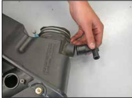
18. Remove the clamp that secures the crankcase vent and then remove the crankcase vent fitting from the airbox.
