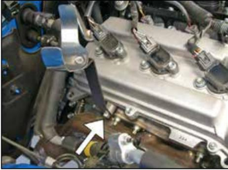
11. Install the tube mounting bracket assembly onto the rear threaded boss on the engine with the provided hardware.
