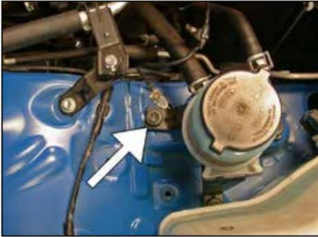
12. Remove the power steering reservoir mounting bolt shown.
