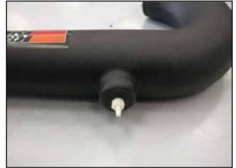
24. Install the supplied 1/4" npt fitting into the K&N intake tube as shown.
