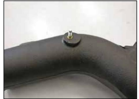
25. Install the engine cover mounting stud into the K&N intake tube as shown, this stud was removed in step #19.
