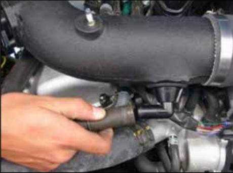
29. Install the crankcase vent hose onto the vent fitting and secure with the factory clamp.
