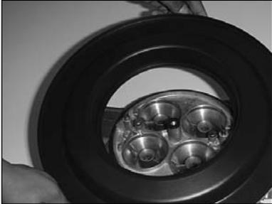
3) Place K&N base plate onto carburetor.
