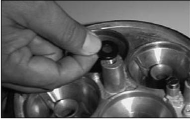
2) Apply spacer onto carburetor center post.
