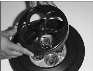
4) Place the K&N Flow Control Stub Stack onto base plate. **NOTE:** make sure the spacer remains in place when placing the stub stack onto the carb post.
