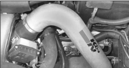
19. Fit the K&N Typhoon intake tube into the silicone hose using the hose clamp supplied. Do not fully tighten yet!
