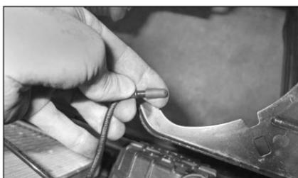
9. Fit the supplied rubber cap plug over the end of the vacuum pipe as shown.
