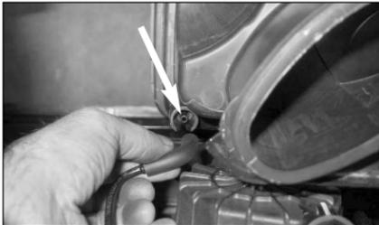
7. Remove the vacuum pipe from the top of the resonator box.
