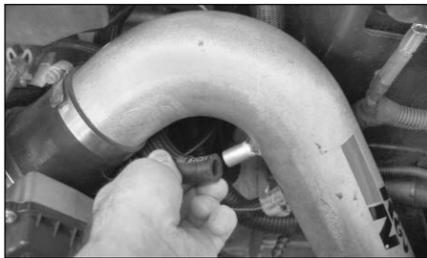
24. Fit the breather hose onto the vent on the K&N Typhoon intake tube as shown.
