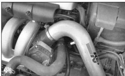
26. Align the intake tube assembly for best fit & clearance, then, firmly tighten all the clamps & hardware connections.
