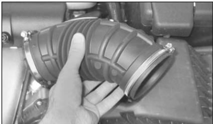
3. Unclip and remove the intake hose from between the throttle body & air box assembly.
