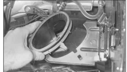
12. Unclip & remove the top of the resonator box from the support bracket.
