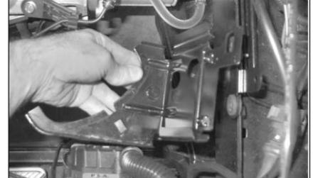
14. Unbolt & remove the main air box support bracket from the vehicle as shown.
