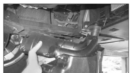
13. Unclip & remove the complete resonator box assembly from the vehicle as shown.
