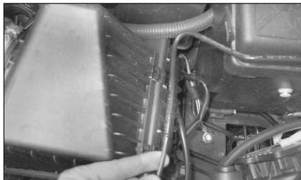
5. Unclip the vacuum pipe from the right side of the air box. Secure the vacuum pipe to the hood release cable using a cable tie supplied.
