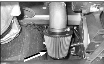
21. From underneath the vehicle fit the filter onto the K&N Typhoon intake tube using the hose clamp supplied.
