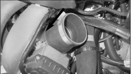
18. Fit the silicone stepped hose onto the throttle body & secure using the hose clamp supplied.
