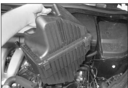
6. Carefully pull the air box assembly from its mountings & remove the assembly from the vehicle.
