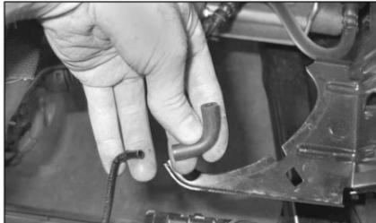
8. Remove the rubber elbow hose from the vacuum pipe as shown.
