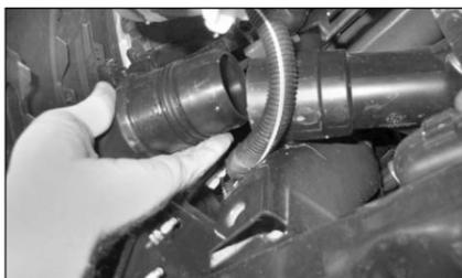
11. From behind the left hand bumper area unclip & remove the intake pipe from the resonator box feed pipe.
