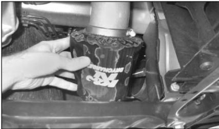
22. Fit the drycharger onto the filter.
