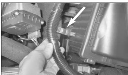
4. Unclip the auxiliary air pump feed pipe from the left hand side of the air box assembly.
