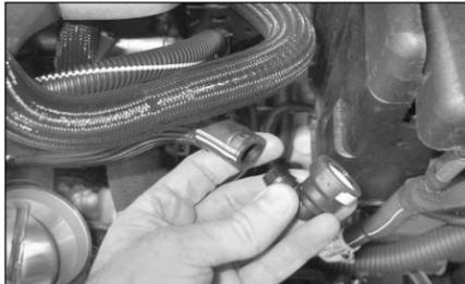
23. Unclip & remove the plastic angled vent from the original breather hose.
