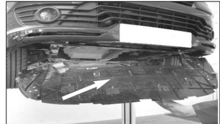
27. Refit the undertray to the underside of the vehicle.
