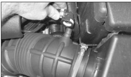
2. Push the tab to unclip, then, remove the breather hose from the side of the intake hose.
