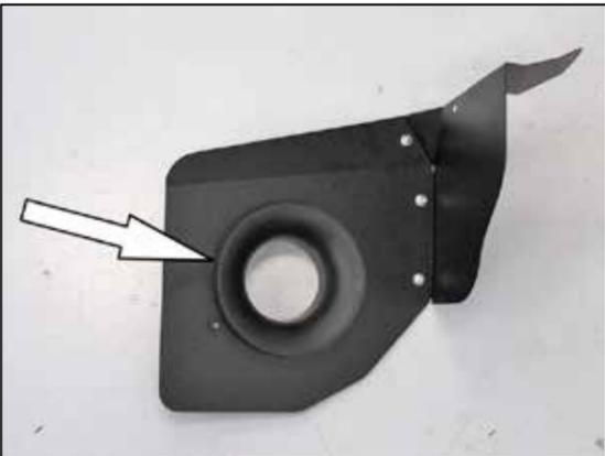
10. Install the filter adapter into the heat shield using the provided hardware.
