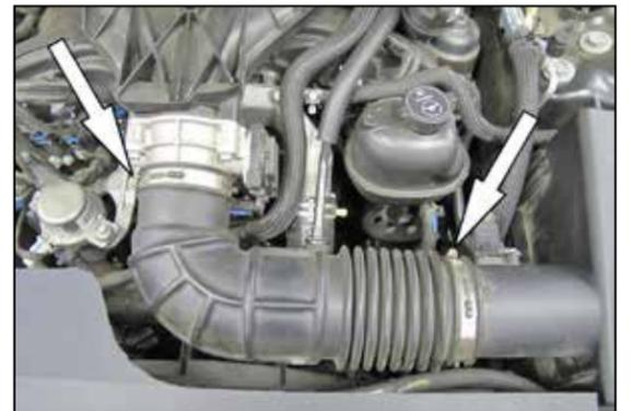
5. Loosen the hose clamps securing the intake tube to the throttle body and air filter housing, then remove the intake tube and crank case vent from the vehicle.
