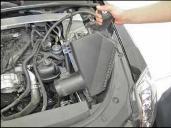
8. Pull up the coolant hoses from the air box and then remove the air box from the vehicle.
