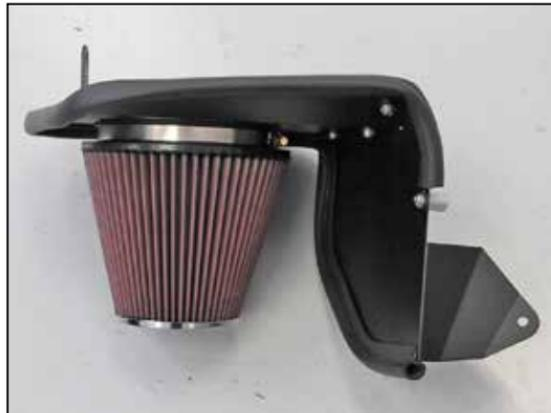
14. Install the K&N® air filter onto the filter adapter and secure with the provided hose clamp.
