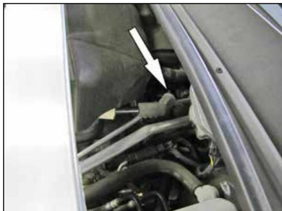
4. Disconnect the crank case vent tube coupler from the rear of the driver's side valve cover.
