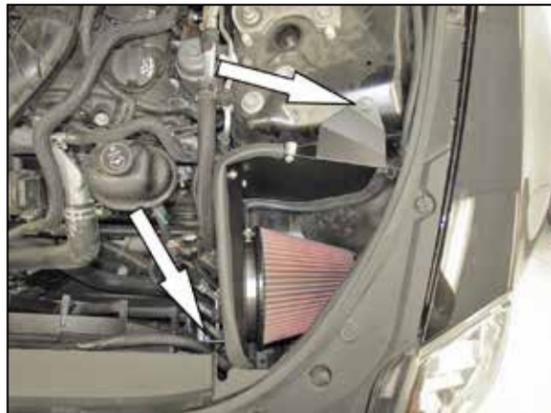
16. Set the heat shield assembly into position and secure it the fan shroud and inner fender with the factory bolts.
