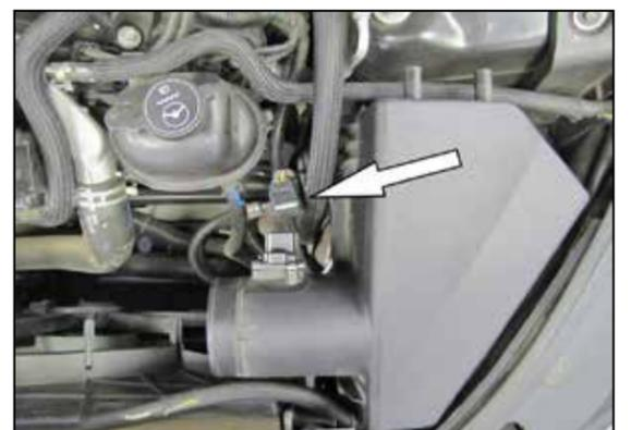
6. Disconnect the mass air sensor electrical connection.
