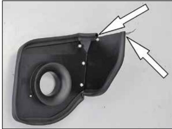
13. Install the provided edge trim onto the heat shield as shown.
