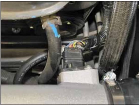
26. Reconnect the mass air sensor electrical connection.
