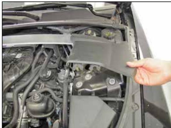
3. Lift up the strut tower cover to unhook it from the holding pins and then remove the cover.
