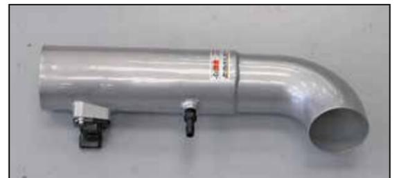
21. Install the provided crank case vent into the K&N® intake tube as shown. **NOTE: Plastic NPT fittings are easy to cross thread. Install the vent fitting "hand" tight, then turn it two complete turns with a wrench.**
