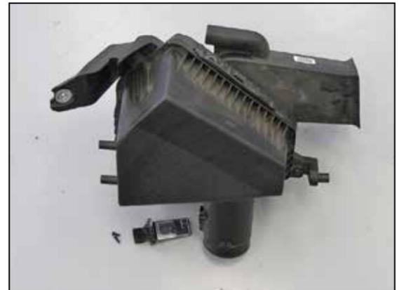
19. Remove the mass air sensor from the factory air box.
