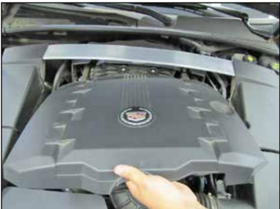
2. Remove the oil fill cap and then lift off the engine cover. Reinstall the oil cap after the engine cover has been removed.
