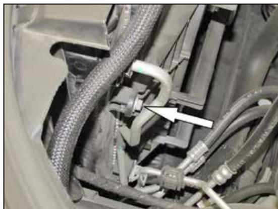
15. Remove the fan shroud mounting bolt shown. **NOTE: This bolt will be reused in the next step.**
