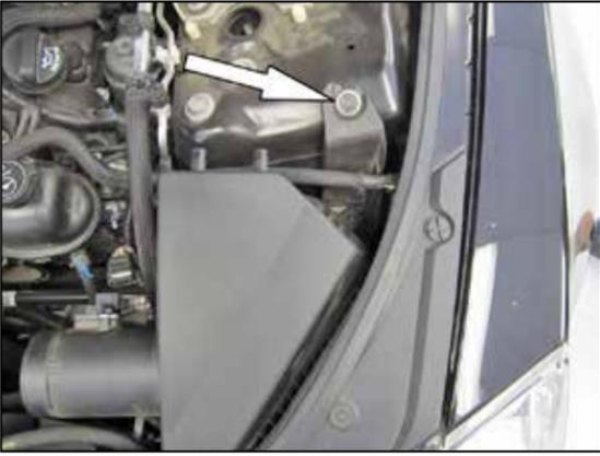
7. Remove the bolt securing the factory air box to the inner fender.
