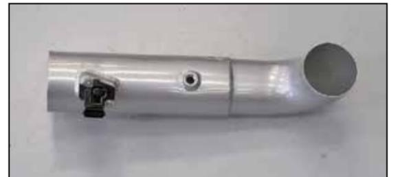
20. Install the mass air sensor into the K&N® intake tube and secure with the provided hardware.
