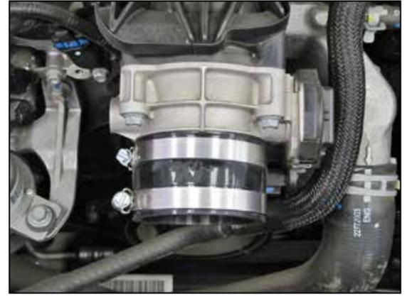
17. Install the provided hose (08434) onto the throttle body and secure with the provided hose clamps.
