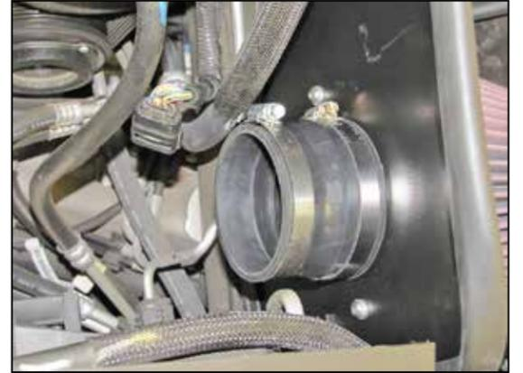
18. Install the provided hose (08051) onto the filter adapter and secure with the provided hose clamps.
