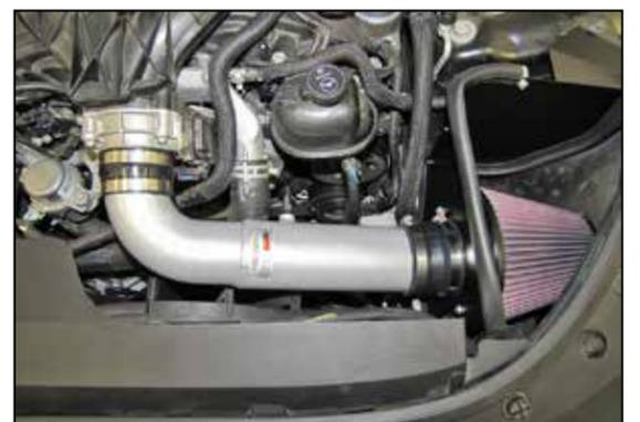
22. Install the K&N® intake tube into the hose at the filter adapter and then into the hose on the throttle body, align the tube for proper fit and then secure with the provided hose clamps.
