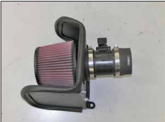
14. Install hose (084031) onto mass air housing and secure with provided hose clamp as shown.
