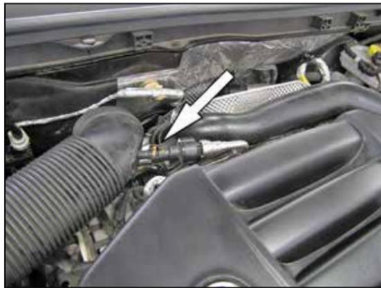
3. Release locking clip and remove crank case vent line from intake tube.
