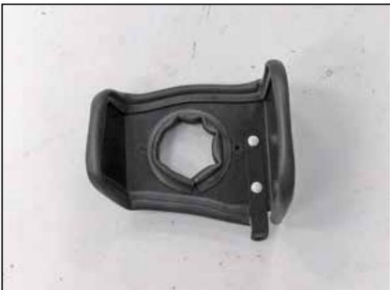
11. Install the 13" length of edge trim into opening of heat shield then the 44" length of edge trim onto heat shield as shown.
