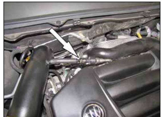
21. Reconnect crankcase vent line as shown.
