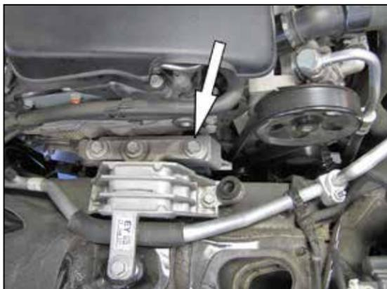
15. Remove forward motor mount bolt shown. **NOTE: Bolt will be reused.**
