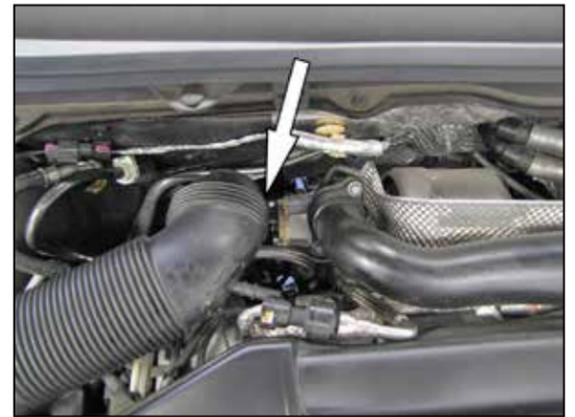
5. Loosen the hose clamp that secures the intake tube to the turbo and remove the intake tube.
