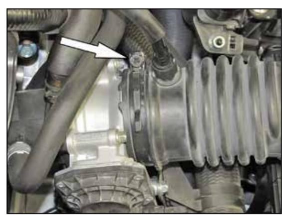
5. Loosen the hose clamp securing the factory intake hose to the throttle body.
