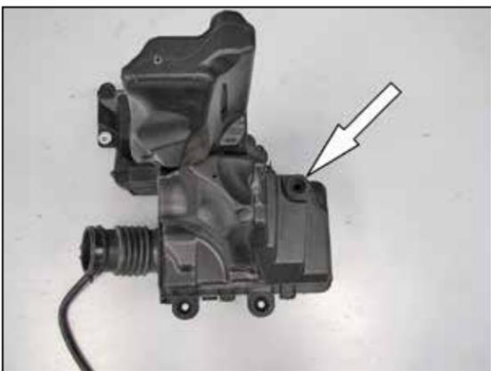
10. Remove the mounting grommet shown from the factory air box.
