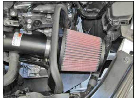
21. Install the filter hose clamp onto the intake tube and then install the filter onto the tube. Reinstall the clamp onto the filter and secure the filter onto the intake tube.
