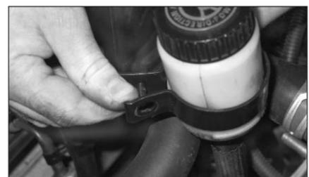
13. Remove the nut securing the PAS reservoir to the mounting bracket. Remove the bracket from the vehicle.
