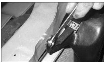
8. Remove the nuts securing the resonator assembly to the slam panel.
