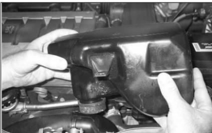
2. Unscrew and remove the upper resonator box from the vehicle.
