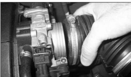
3. Unclip and remove the intake hose from the throttle body.
