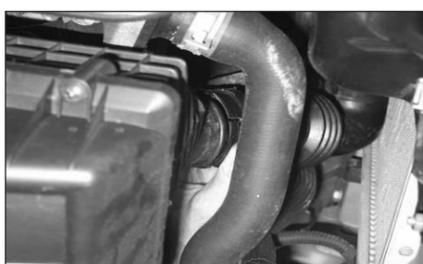
5. Unclip & remove the resonator pipe from the base of the air box assembly.
