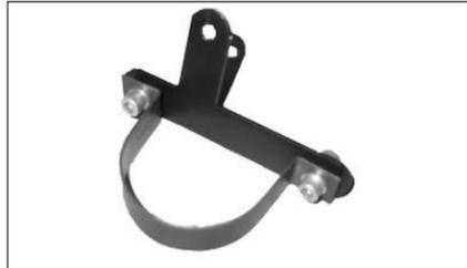
16. Assemble the 'T' bracket and the 'U' bracket using the allen head bolts, small flat washers and nylock nuts supplied as shown. Do not fully tighten at this moment.
