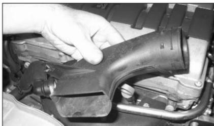
7. Remove the nut securing the intake scoop to the slam panel. Carefully unclip and remove the scoop from the vehicle.
