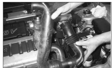
11. Carefully manoeuvre the resonator box assembly from the vehicle.
