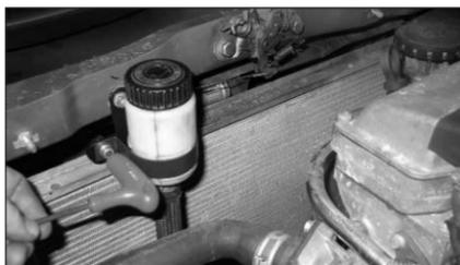
18. Secure the PAS reservoir to the bracket assembly and now fully tighten all connections.
