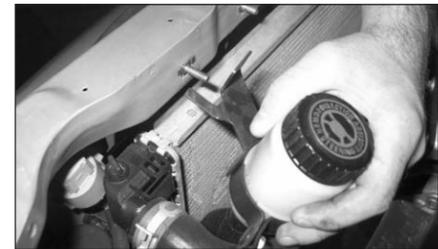
12. Remove the nut/ bolt securing the PAS (Power Assisted Steering) reservoir to the slam panel.
