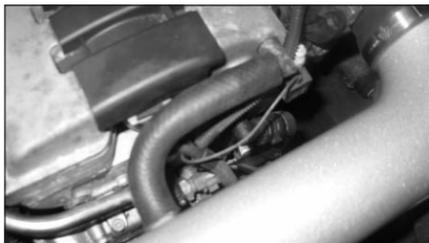
23. Fit the new vent hose to the vent adaptor located on the cam cover and the new intake tube. **Note:** It might be necessary to trim the new hose to suit.
