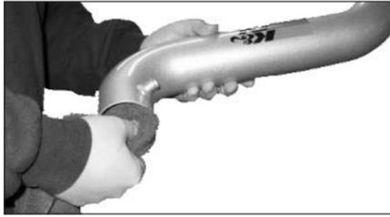
20. Before installing the new tube, clean the inside of the new intake tube out with water and a towel.
