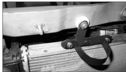
17. Secure the new bracket assembly to the front slam panel using the plastic spacer and one of the nuts/ bolts removed earlier. The spacer comes between the slam panel and the bracket.
