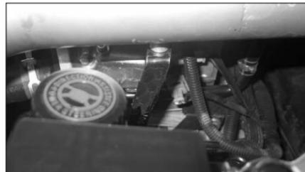
22. Secure the mounting bracket to the threaded boss on the underside of the Typhoon tube using a short bolt and wave washer supplied.
