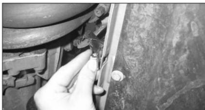
10. Remove the bolt securing the resonator box assembly to the lower cross member.
