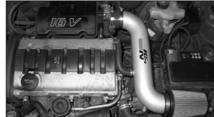
26. Reconnect the negative battery cable. Double check that everything is tight and properly positioned before starting the vehicle.
