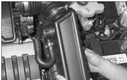
6. Carefully lift the complete air box assembly out of its lower mountings and remove the assembly from the vehicle.
