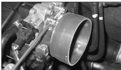
19. Secure the stepped silicone adaptor hose to the throttle housing using the #275 barrel clamp supplied.
