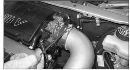
25. Adjust the Typhoon tube for best fit and clearance. Now fully tighten all the hardware.
