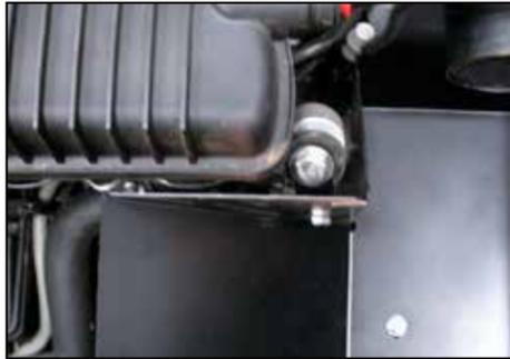
32. Secure the "L" bracket to the threaded insert as shown.
