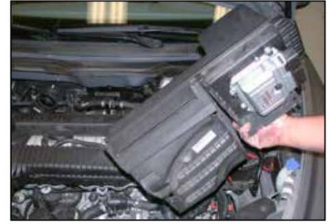
18. Pull firmly upwards to release the air box from the rubber mounting grommets, then carefully slide the air box towards the battery side of the vehicle; slowly remove from vehicle.
