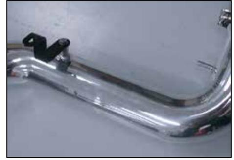
35. Install the "Z" bracket to the intake tube as shown.
