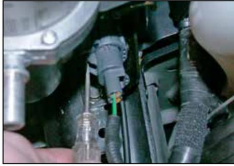
16. Disconnect the EVAP pump electrical connection by inserting a small flat blade screwdriver and depressing the locking clip while pulling the connector away from the harness.
