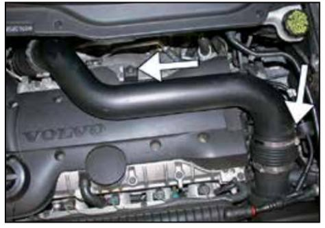
2. Remove the two bolts that secure the stock intake tube.
