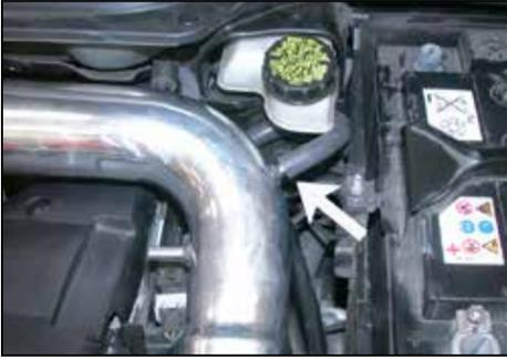
42. Connect the other end of the EVAP recirculation line hose to the vent tube on the intake tube as shown.
