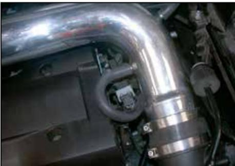
44. Route the hose underneath the intake tube and connect it to the vent tube on the intake tube as shown.
