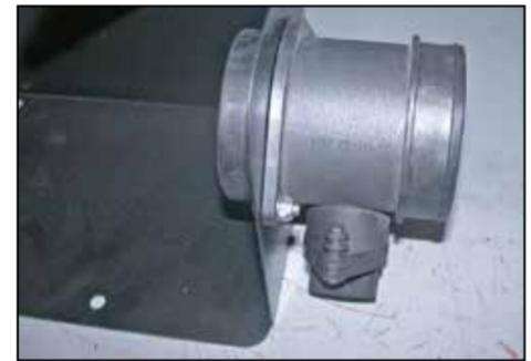
21. Install the mass air sensor onto the heat shield and secure it with the provided hardware.
