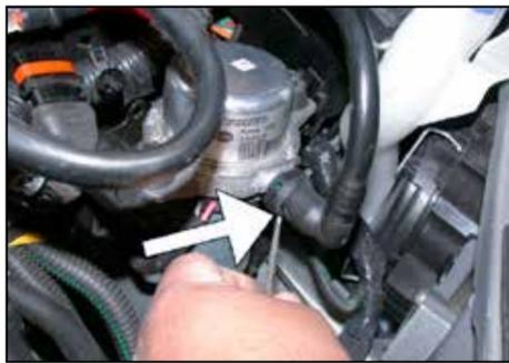
15. Depress the locking tab on the EVAP hose to release from the EVAP pump.
