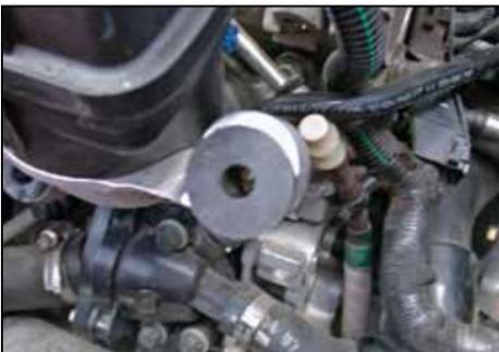
28. Install the threaded insert into the air box mounting hole from step 26.
