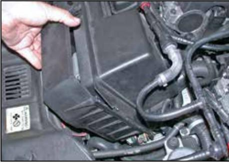
8. Lift and remove the plastic ECM cover from the air box.
