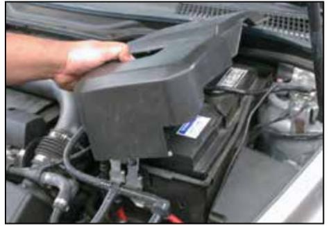
1. Turn the ignition OFF and disconnect the vehicle's negative battery cable by first removing the battery cover as shown.
