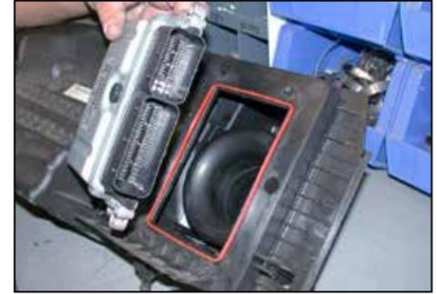
19. Remove the four bolts that secure the ECM to the air box using a T30 torx.
