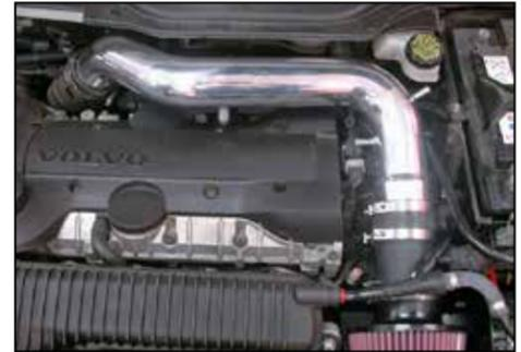
38. Install the K&N® intake tube into the stock intake hose, attaching the other end onto the mass air sensor. Secure the intake tube to the stock hose with the stock hose clamp and secure the intake tube to the mass air sensor with the provided hose clamp.
