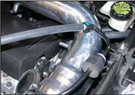
43. Insert the carbon filter vacuum hose onto the stock crank case hose as shown.
