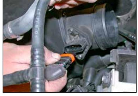
5. Disconnect the mass air sensor electrical connection as shown.
