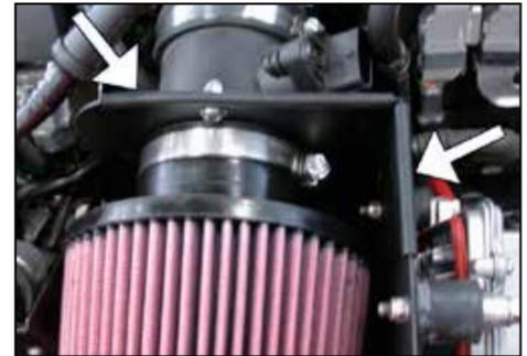
37. Using the supplied edge trim, cut to size and fit over the heat shield as shown.
