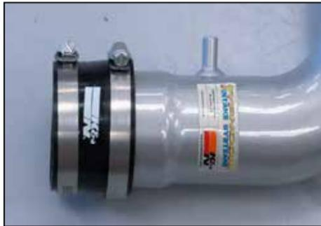
34. Install the silicone hose and provided hose clamps to the K&N® intake tube.
