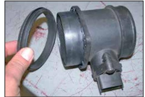
20. Remove the mass air sensor O-ring from the mass air sensor.
