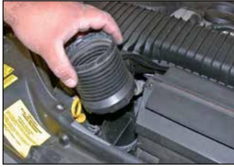
13. Twist and remove the accordion hose from the lower air inlet duct as shown.
