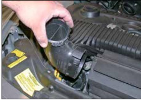
14. Pull upwards to remove the lower air inlet duct from the air box as shown.
