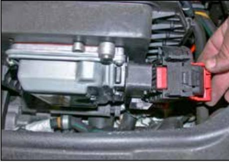
9. Depress the release tabs on the upper and lower electrical harness and disconnect from the ECM as shown.
