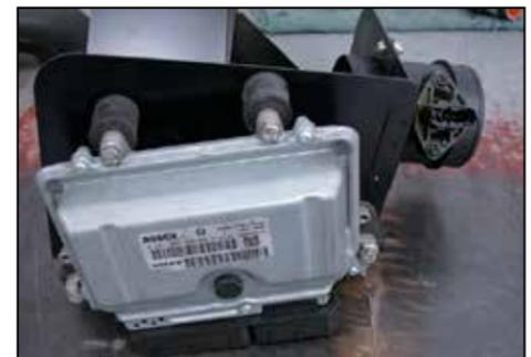
23. Mount the ECM onto the heat shield with the provided hardware as shown.
