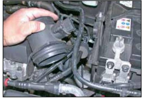
6. Using a Torx T25, remove the two bolts that secure the mass air sensor to the air box and remove from the vehicle.
