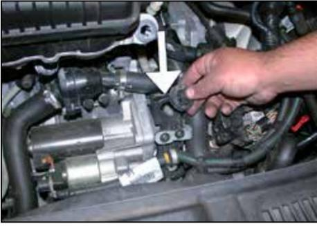
24. Remove the large air box mounting grommet from the vehicle.
