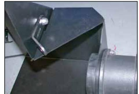
22. Install the "L" bracket onto the heat shield and secure it with the provided hardware.
