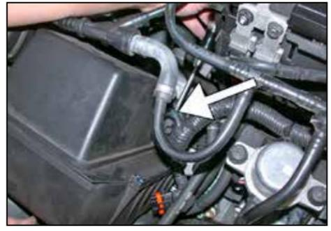
7. Remove the bolt that secures the main wiring harness to the air box, then unclip the harness from the air box.
