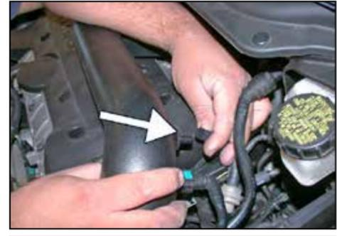
4. Lift slightly and remove the EVAP recirculation line. Remove the carbon filter vacuum hose by depressing the two locking tabs as shown, then remove the intake tube from vehicle.
