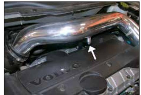
39. Secure the intake tube to the bracket with the provided hardware as shown.
