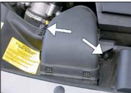
12. Loosen and remove the two screws that secure the upper air inlet duct, then remove from vehicle.
