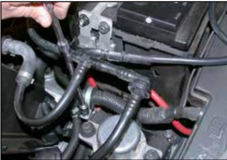
10. Loosen and remove the Delphi clamp bolt that secures the main wiring harness to the EVAP pump.
