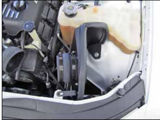
13. Set the heat shield assembly into position in the engine bay so the inserted nut passes into the air box mounting hole in the inner fender. Do not secure the heat shield at this time.
