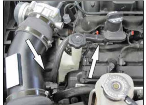
21. Install the assembled vent hose onto the fitting installed in the K&N® intake tube and then attach the open end to the valve cover port.
