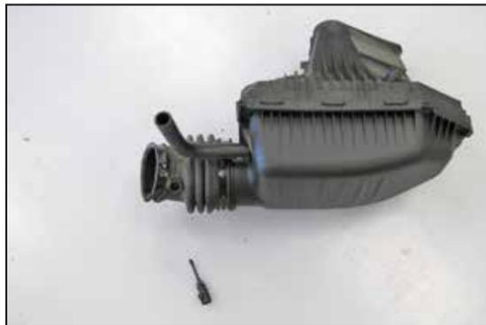
16. Remove the inlet air temperature sensor from the factory intake tube as shown.
