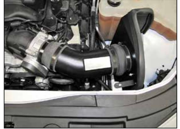
18. Install the K&N® intake tube into the silicone hump hose and then into the silicone step hose at the throttle body. Align the intake tube and heat shield for proper fit and then secure the intake tube with the provided hose clamps and the heat shield bracket with the factory air box retaining bolt removed in an earlier step.
