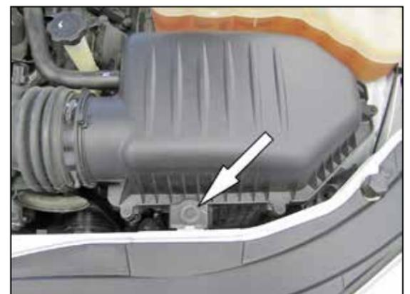
6. Remove the bolt which secures the air box to the core support.
