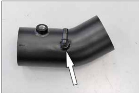
15. Install the provided 90° NPT vent fitting into the K&N® intake tube as shown.
