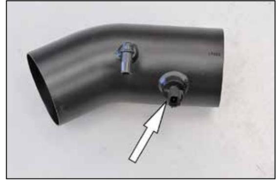
17. Install the inlet air temperature sensor into the K&N® intake tube as shown.
