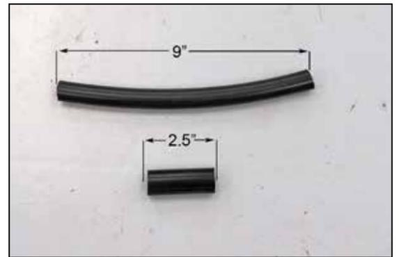
19. Cut the provided 1/2" silicone vent hose to a length of 9" long, and cut the 5/8" vent line to a length of 2.5" long.
