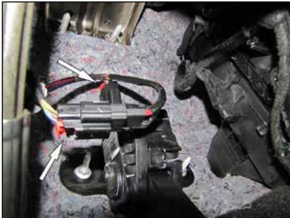
3. Connect the K&N® throttle wiring harness to the throttle pedal and connect the factory wiring harness to the K&N® wiring harness.
