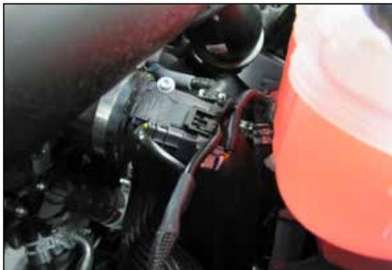
2. Disconnect the TIP sensor electrical connection and then connect the K&N® wiring harness connectors to the TIP sensor and to the factory harness.
