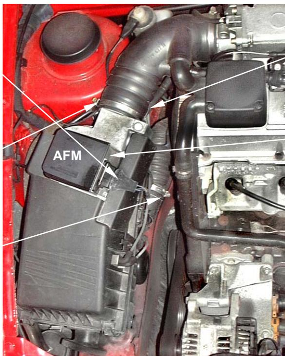
**4.** Remove the hot air control valve vacuum hose from the 'T' piece and fit the rubber cap to the end of the 'T' piece. (This will prevent an air leak).
