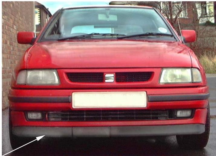
Pierce / drill two 3mm holes in the front lower spoiler trim, secure the rubber intake scoop to the spoiler using 2 medium plastic ties. Insert the flexi cold air hose into the scoop, secure the rear of the scoop using a long plastic tie supplied.
