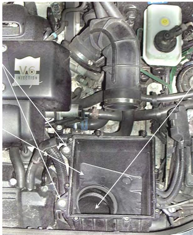
**3.** Remove the 2 bolts securing the intake tube to the chassis leg and remove the tube from the car. (It may be necessary to remove the air box mounting bracket to remove the intake tube).
