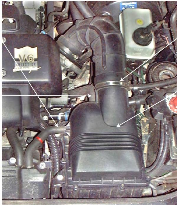
**3.** Unclip and remove the intake hose from the air box lid.
