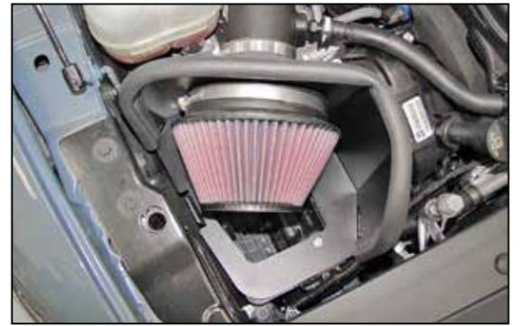
18. Install the K&N® air filter onto the filter adapter and secure with the provided hose clamp.
