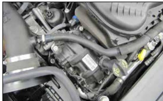
17. Install the crank case quick connect fitting into the factory crank case vent hose and connect it to the fitting installed into the K&N® intake tube.
