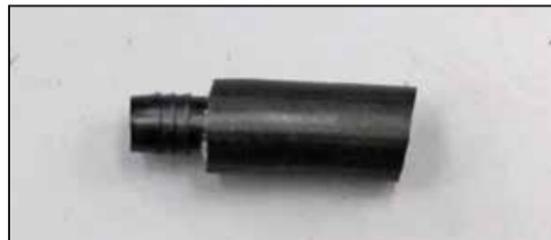
14. Install the provided hose mender into the section of crank case vent hose provided.
