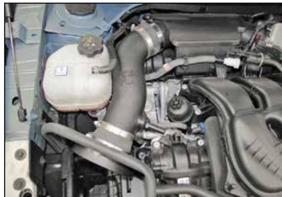
16. Install the K&N® intake tube into the coupling hose at the plenum, align the coupling hose at the filter adapter and then adjust the tube for best fit and tighten all of the hose clamps.
