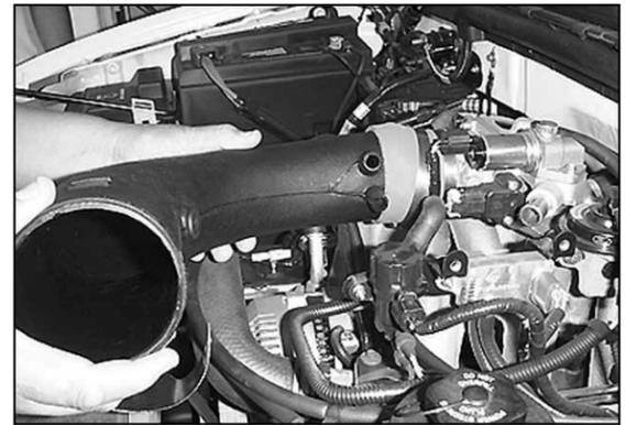
19. Install the intake tube into the small silicone hose and tighten clamp.
