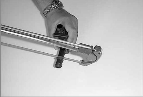
21. On models with 4.6L engines, in some isolated instances where a whistling noise may exist. Cut the flange of the air bypass valve just past the last barb as shown. Reinstall the air bypass valve, attaching it to the appropriate fitting on the intake tube using the 3/4" id hose and hose clamps provided.
