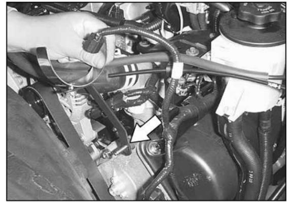
17. Install the saddle bracket assembly onto the protruding stud as shown, secure into place using the hardware provided.
