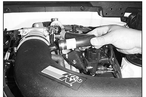
20b. On vehicles equipped with a 4.6L engine, attach the provided 5/8" idle air by-pass vent hose onto the appropriate fitting on the intake tube, trim for proper fitment to prevent the hose from developing a kink and attach the open end to the idle air by-pass valve.
