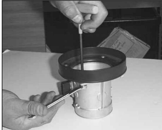
13. Attach the mass air adapter to the mass air sensor using the gasket and hardware provided as shown above.
