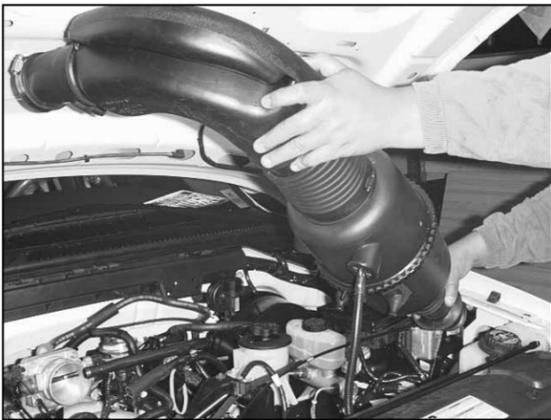
8. Remove the entire stock air intake assembly from the vehicle.
