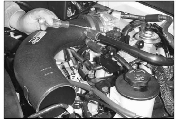
20a. On models with 5.4L engines, install the idle air control and crankcase vent hose onto the appropriate fittings on the intake tube, secure with the hose clamps provided.
