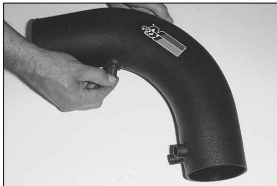
15. Using the grommet provided, install the air temperature sensor into the intake tube.
