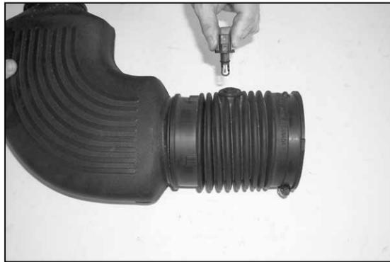
14. Remove the air temp. sensor from stock air intake tube as shown.
