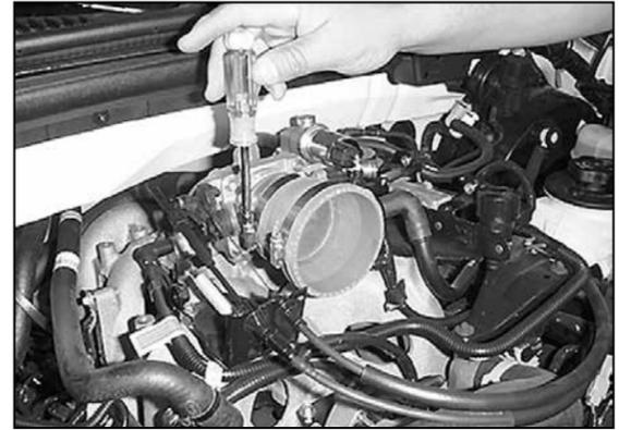
18. Using the hose clamp provided, attach the small silicone hose to the throttle body.
