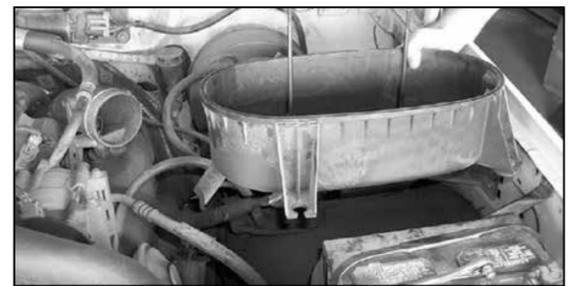
7. Pull firmly upwards to release the lower air cleaner assembly from the retaining grommets, then remove as shown.
