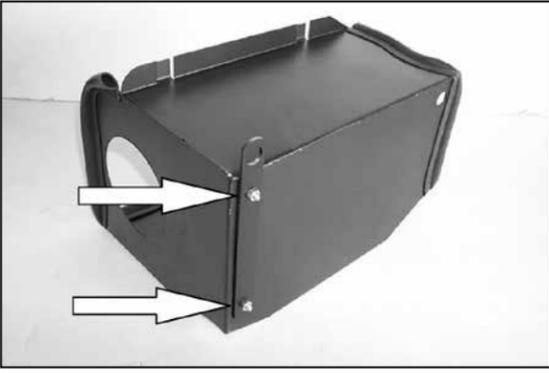
10. Using the provided hardware, install the straight bracket onto the bottom of the K&N® heat shield as shown.
