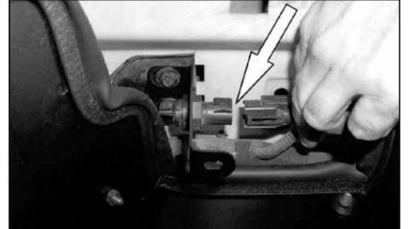
21. Reconnect the air temperature sensor electrical connection as shown.
