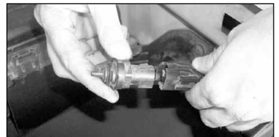
8. Using a small flat blade screwdriver, release the Air Temperature Sensor retaining clips, then disconnect the electrical connection as shown.
