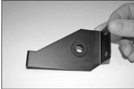
17a. Vehicles that come with twist in air temp sensor, install grommet (08167) into air filter support bracket as shown.
