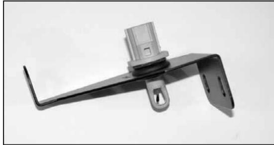
17b. Vehicles that come with twist in air temp sensor, install sensor into air filter support bracket as shown.
