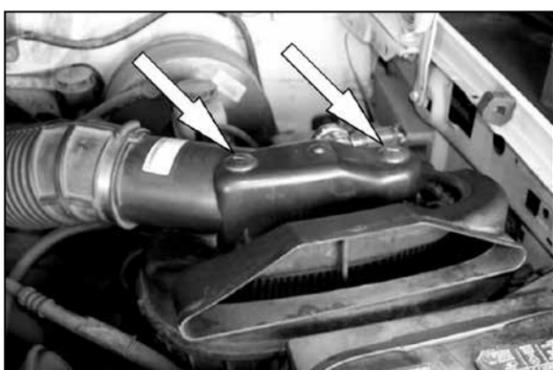
3. Loosen the screws that secure the air cleaner top as shown. (see arrows)
