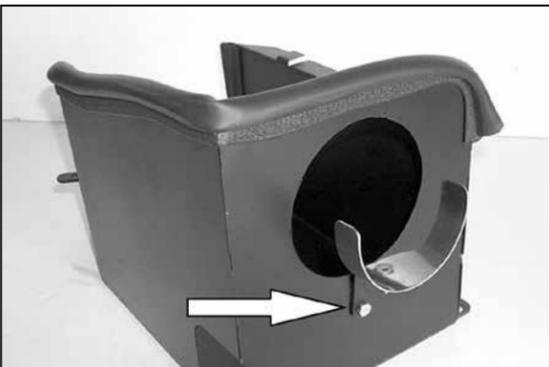
13. Install the saddle bracket assembly onto the K&N® heat shield using the provided hardware as shown.
