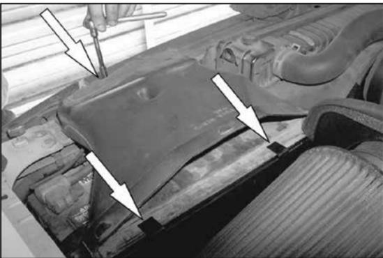
29. Slide the air inlet duct into the tabs on the K&N® intake tube as shown, then, secure the air inlet duct to the original mounting point with the original hex bolt removed in step 2.
