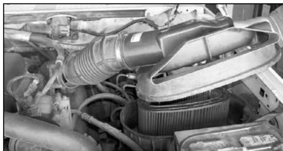
4. Loosen the hose clamp at the turbo inlet tube, then remove the upper air cleaner assembly as shown.
