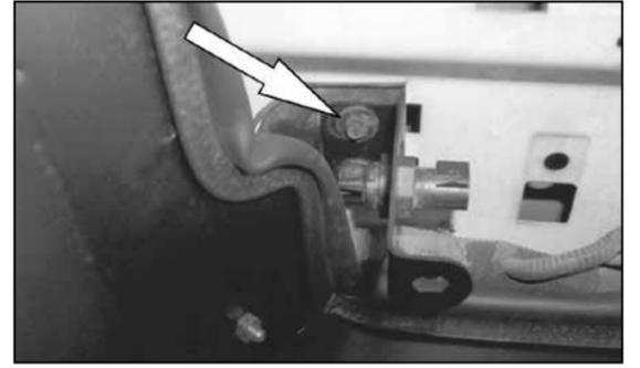
20. Install the air filter support bracket onto the fuse box support bracket using the bolts removed in step 15.
