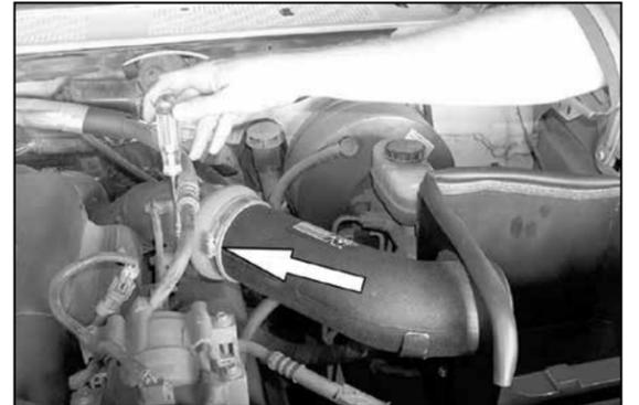
22. Install the K&N® intake tube onto the turbo inlet tube and secure the hump hose with the provided hose clamp.
