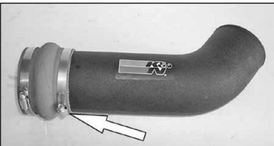
14. Install the silicone hump hose onto the K&N® intake tube as shown and secure with the provided hose clamp.
