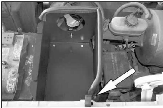
19. Install the K&N® heat shield assembly and push the rubber grommets onto the stock locating pins, then, secure the "L" bracket to the original air cleaner rubber mounting stud using the provided washer and nylock nut.
