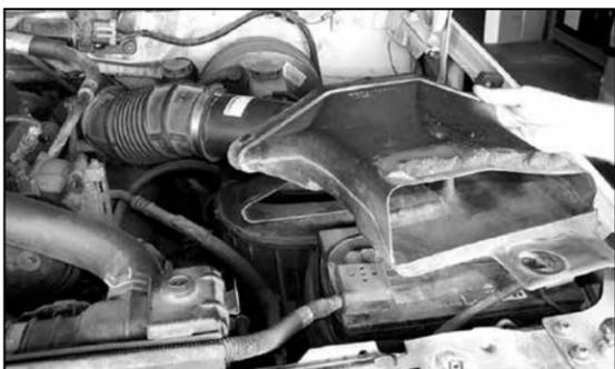
2. Loosen and remove the bolt on the radiator core support, then remove the air inlet duct as shown.
