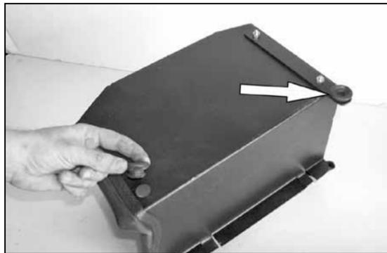
18. Install the stock rubber grommets from the lower air cleaner assembly into the K&N® heat shield assembly as shown.
