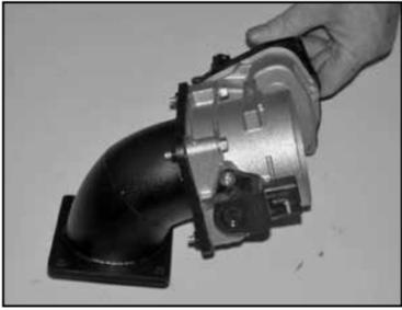
12. Using the bolts removed in step #10, secure the throttle body to the K&N® throttle body adapter with the gasket as shown.
