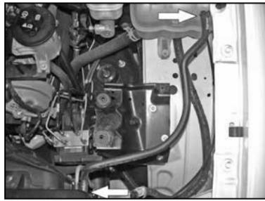
17a. Loosen the coolant recovery hose, hose clamps, and then remove the factory recovery hose shown. Be sure to catch any coolant, which flows out of the radiator during hose removal.
