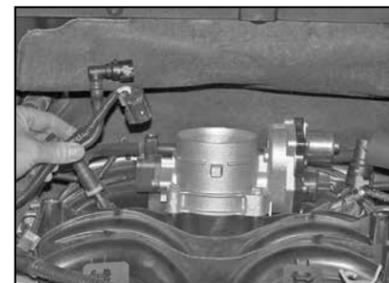
9. Disconnect the TPS sensor electrical connection from the throttle body.
