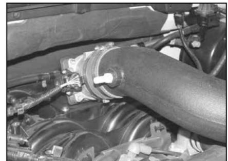
27. Install the K&N® intake tube into the silicone hose and then tighten the provided hose clamp.
