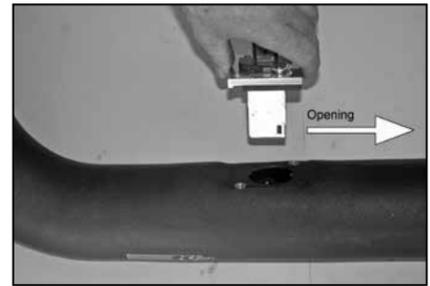
22. Install the mass air sensor assembly into the K&N® intake tube.
