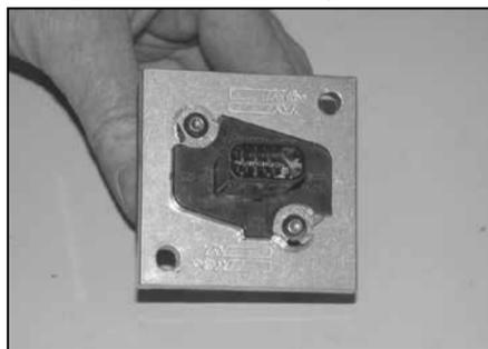
21. Install the mass air sensor into the K&N® mass air adapter as shown and secure with the provided hardware.
