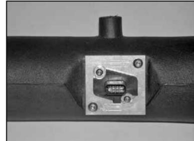
23. Secure the mass air sensor assembly onto the K&N® intake tube with the provided hardware as shown.
