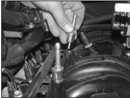
30b. Re-install the factory air box mounting studs with the provided spacers as shown.
