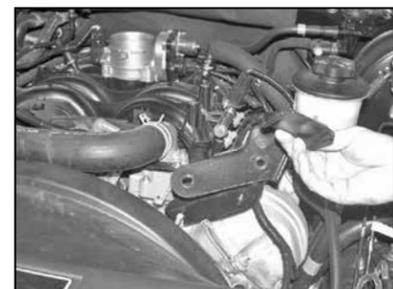
7. On vehicles that are equipped with the intake tube support bracket, remove the two 13mm nuts securing the intake tube support bracket, remove the intake tube support bracket.
