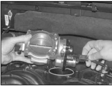
11. Lift the throttle body from the intake manifold and disconnect throttle body motor electrical connection.
