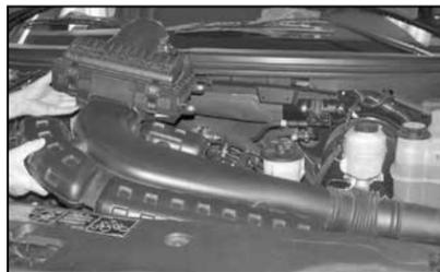
6. Remove the entire intake tube & air filter assembly from the vehicle.
