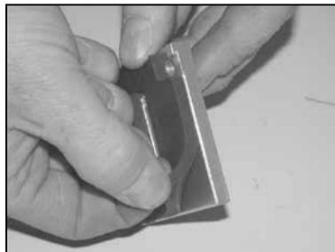
20. Install the provided gasket onto the K&N® mass air adapter as shown; sticky side down.
