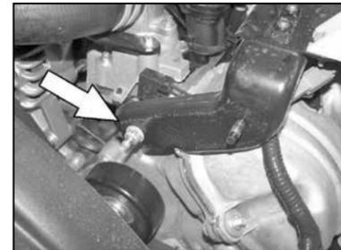
8. On vehicles that are equipped with the intake tube support bracket, reinstall one of the 13mm nuts removed in step #7 onto the lower mounting stud and tighten.
