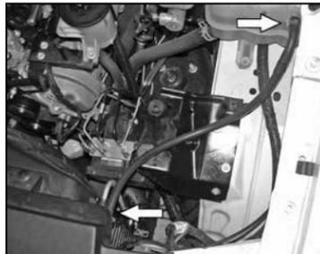
17b. Install the supplied coolant recovery hose and secure with the provided hose clamps.
