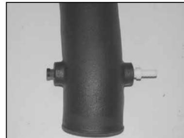
24a. On vehicles that are equipped with only one vent line, install the provided NPT plug as shown.
