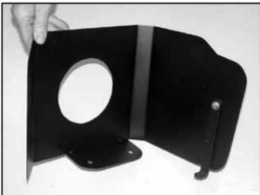
15. Install the "L" bracket (#070026) onto the heatshield with the provided hardware as shown.
