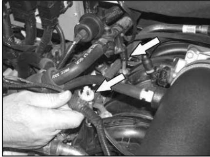
30c. Re-install the heater control valve and wiring harness mounting clips onto the air box mounting studs as shown.
