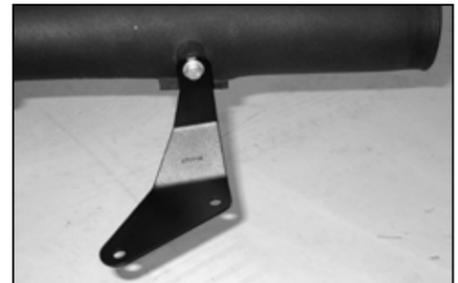
25. Install the tube mounting bracket (070118) onto the K&N® intake tube as shown with the provided hardware.
