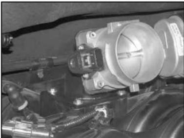
13. Install the throttle body assembly onto the intake manifold with the hardware provided as shown.
