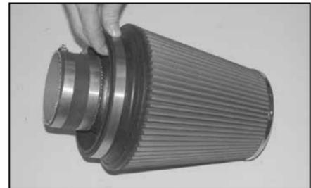
33. Install the adapter assembly into the K&N® air filter as shown.
