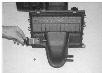
19. Remove the two screws that secure the mass air sensor to the air box with the provided wrench, then remove the mass air sensor.
