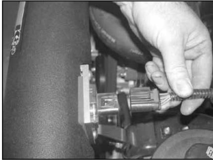
31. Reconnect the mass air sensor electrical connection.
