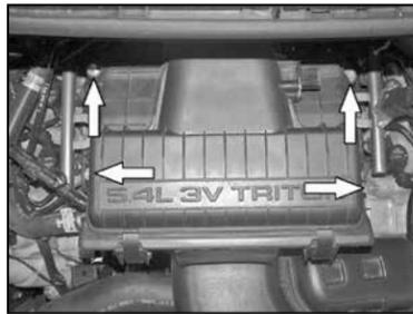
4. Remove the four air box mounting bolts shown with a 10mm socket.
