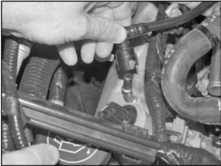
29. Unlock the crank case vent hose and remove the hose from the valve cover.
