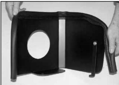
16. Install the edge trim onto the heatshield as shown.
