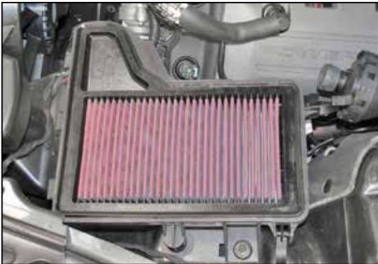
10. Install the K&N® air filter into the lower air filter housing.
