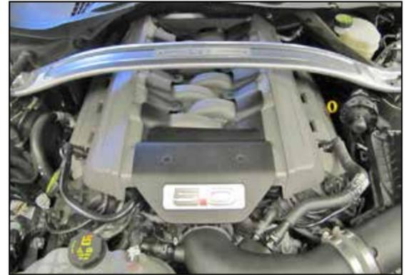
19. Reinstall the Engine cover onto its mounting studs.
