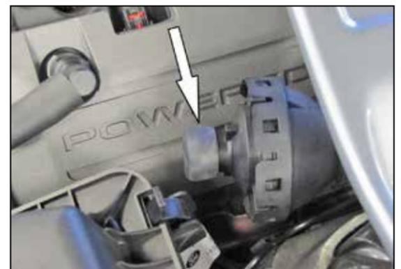
6. Install the provided cap onto the sound drum as shown.
