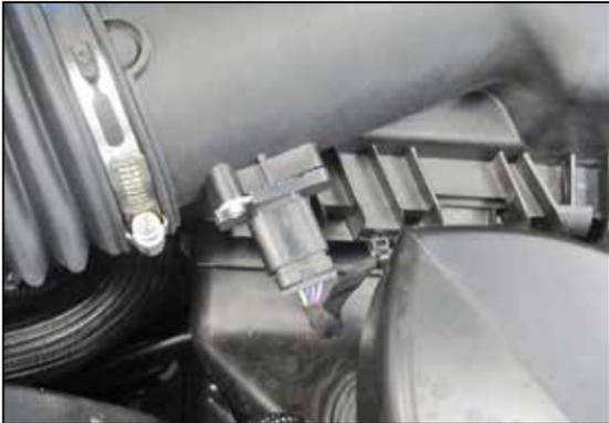
8. Release the red locking tab on the underside of the MAF electrical connector and then disconnect the MAF electrical connection.
