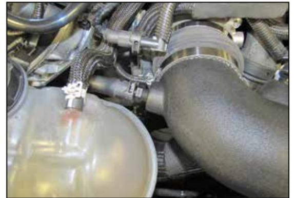
18. Connect the idle by-pass vent line to the quick disconnect fitting installed into the K&N® intake tube as shown.
