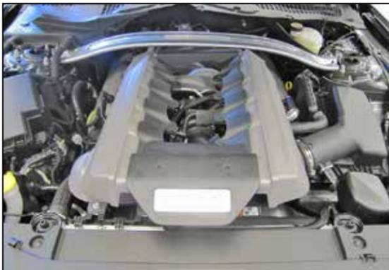
2. Lift up the engine cover to unhook it from its mounts, slide the engine cover from under the strut tower brace and remove it from the vehicle.
