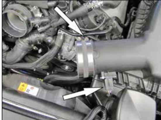
14. Install the provided coupling hose (08563) onto the air filter housing and secure with the provided hose clamp then reconnect the mass air sensor electrical connection.
