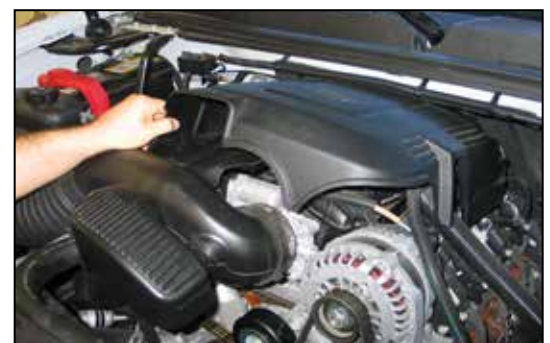
3. Lift up and remove the engine cover from the engine as shown.
