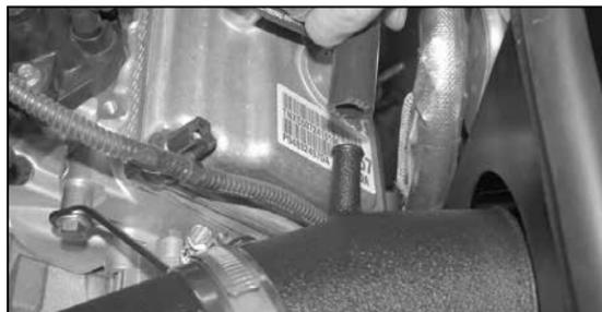
19. Install the provided crank case vent hose onto the vent port on the valve cover then install the vent hose onto the K&N® intake tube.
