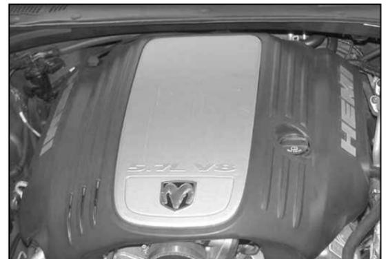
24. Reinstall the engine cover removed in step #2.
