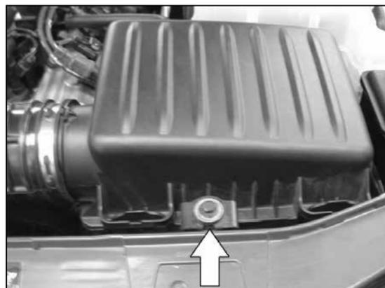
6. Loosen and remove the airbox mounting bolt as shown.
