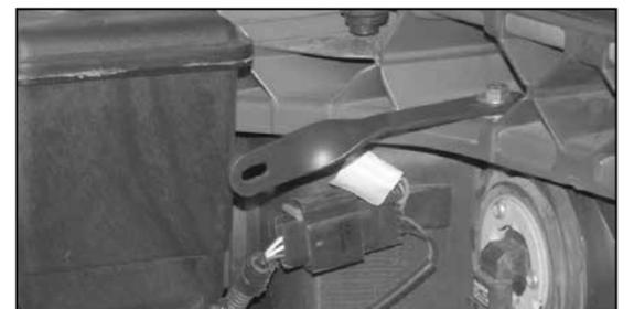
8. Install the twist bracket (070772A) onto the core support using the hardware provided through the existing hole as shown.
