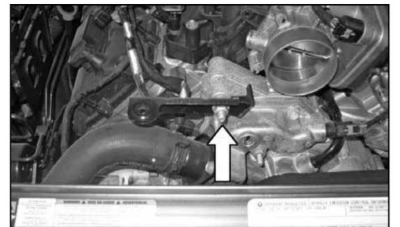
7a. On vehicles equipped with an intake resonator, remove the nut shown that secures the resonator bracket; remove the resonator bracket from the engine.
