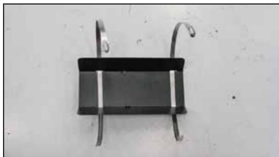
17. Install the two large hose clamps into the air filter housing mounting bracket as shown.
