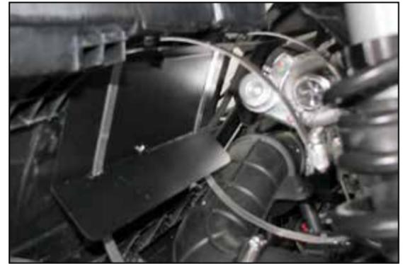
18. Install the air filter mount into the vehicle so that the hose clamp adjusters are on the top and the bolts are off set to the left. Secure the mount with the hardware provided.
