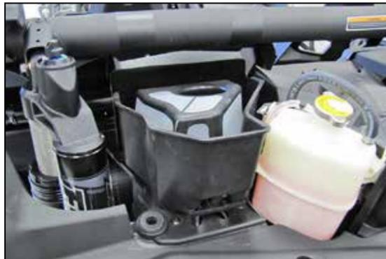
32. Reinstall the clutch filter assembly.
