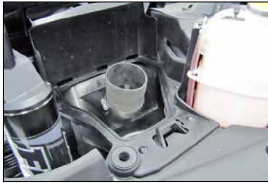
28. Install the fresh air intake hose (08429) onto the Fresh air intake tube. Adjust the tube so that it is tight against the housing, slide the hose down tight against the housing and then secure the hose clamp.
