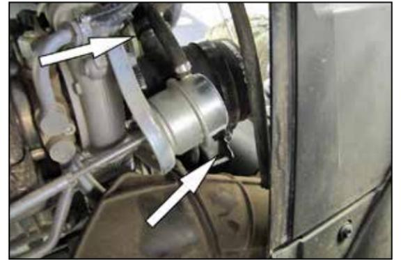
20. Install the K&N intake hose assembly (084103) onto the turbo, rotate the hose so that the crank case vent hose aligns with the fitting installed into the K&N hose. Install the crank case vent hose and secure with the factory hose clamp. Connect the vacuum hose to the fitting installed into the K&N intake hose.
