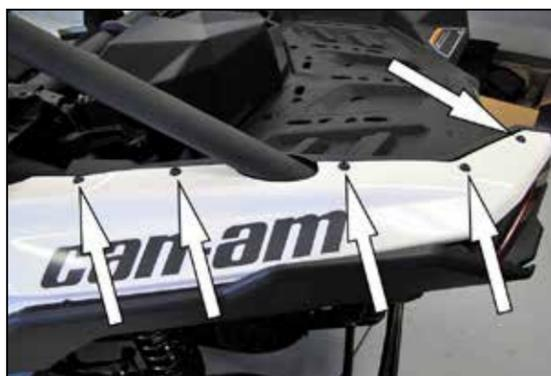
3. Remove the five fasteners and clip nuts securing the top of the fender.
