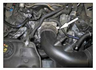
8. Loosen the hose clamp which secures the factory intake tube to the throttle body.
