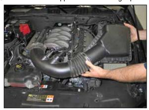
10. Remove the upper air box and intake tube from the vehicle.
