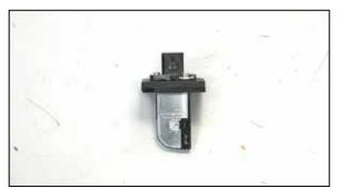
24. Install the mass air sensor into the K&N<sup>®</sup> adapter and secure with the provided hardware.
