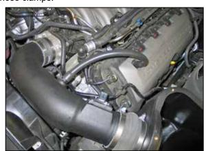
27. Install the crank case vent hose to the fitting on the K&N<sup>®</sup> intake tube and on the valve cover. Vehicles equipped with an EVAP vent line, connect it to the fitting installed in the K&N<sup>®</sup> intake tube.
