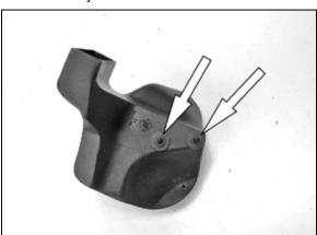
16. Install the air box mounting grommets onto the two mounting studs installed onto the K&N® air box.
