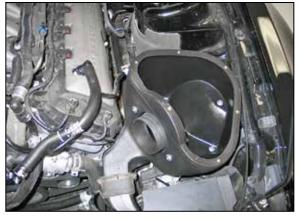
17. Set the K&N<sup>®</sup> air box into the vehicle so that the mounting studs slide into the mounting holes, and then secure with the hardware provided.
