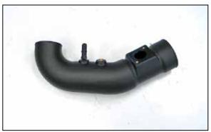
20. Install the Crank case vent fitting into the  $K\&N^{\tiny \circledcirc}$  intake tube as shown.
