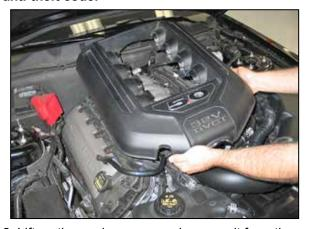
2. Lift up the engine cover and remove it from the vehicle.
