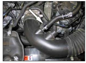
7. Disconnect the crank case vent hose from the factory intake tube and valve cover port and then remove the vent tube from the vehicle.
