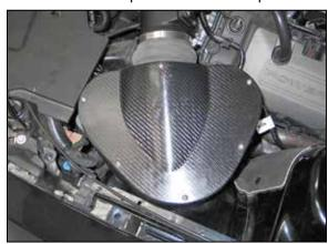
30. Install the K&N® air box lid and secure with the provided hardware.
