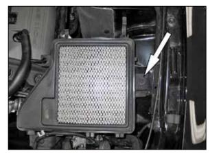
11. Remove the bolt that secures the lower air box to the inner fender.
