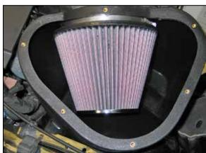
29. Install the K&N® air filter onto the filter adapter and secure with the provided hose clamp.
