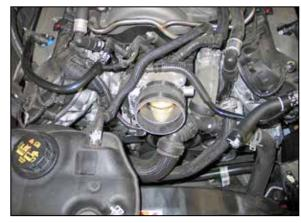
19. Install the provided silicone hose (08497) onto the throttle body and secure with the provided hose clamp.
