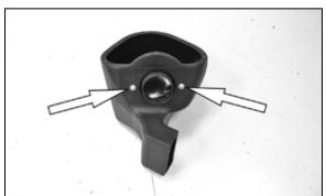
14. Install the filter adapter into the air box and secure with the provided hardware.
