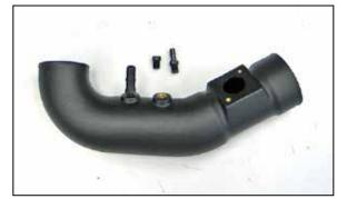
21. On vehicles that have an EVAP vent line attached to the intake tube, install the 3/8" vent fitting into the K&N® intake tube. On vehicles that do not have the EVAP vent line attached to the intake tube, install the npt plug into the intake tube. NOTE: Plastic NPT fittings are easy to cross thread. Install the vent fitting "hand" tight, then turn it two complete turns with a wrench.
