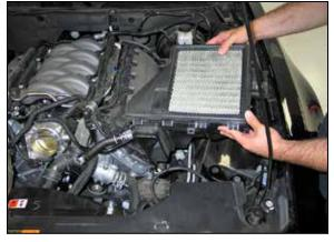
12. Remove the lower air box from the vehicle. NOTE: K&N Engineering, Inc., recommends that customers do not discard factory air intake.
