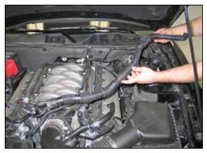
4. Release the clamp which secures engine pulse hose to the intake tube then remove the engine pulse hose from the vehicle.
