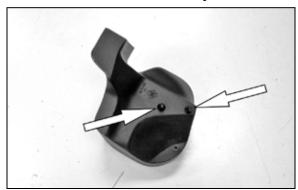
13. Install the two air box mounting studs onto the bottom of the air box and secure with the provided hardware.
