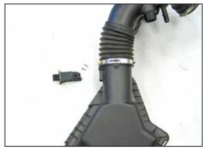
26. Install the K&N® intake tube into the silicone hose at the air box and then into the silicone hose at the throttle body and secure with the provided hose clamps.
