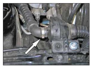
3. Cut the clamp which secures the engine pulse hose to the drum and disconnect the hose from the
