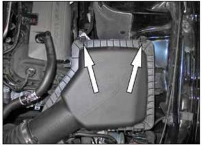
9. Release the two upper air box retaining clips.
