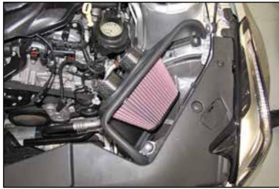
12. Install the heat shield assembly into the vehicle so that the mounting studs insert into the factory air filter housing mounting grommets.
