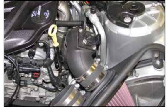
18. Install the driver's side intake tube into the coupler at the turbo and then into the coupler on the filter. Secure the tube with the provided hose clamps.
