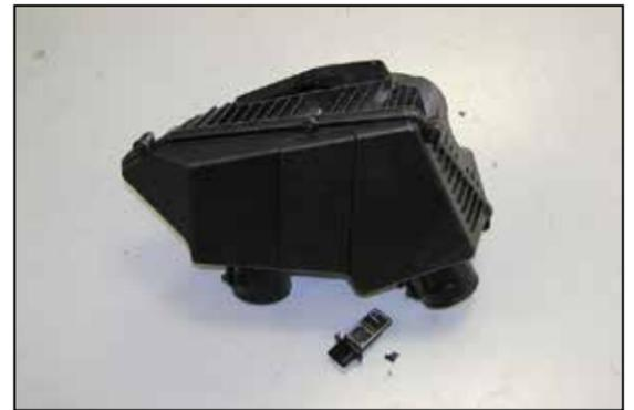
19. Remove the passenger side mass air sensor from the factory air filter housing.
