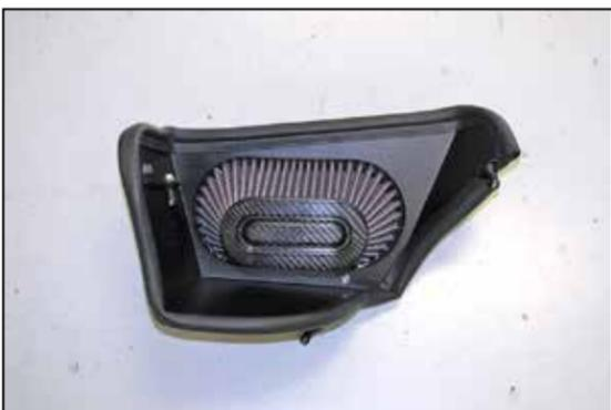
11. Install the K&N® air filter into the heat shield.
