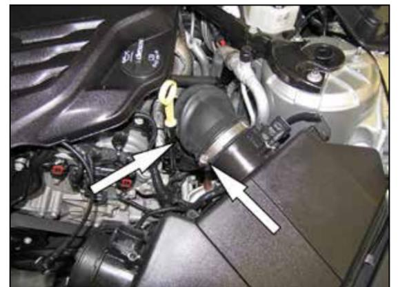
5. Loosen the hose clamps that secure the driver's side factory intake tube and then remove the tube from the vehicle.
