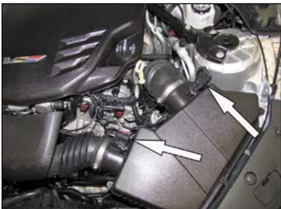
2. Disconnect the mass air sensor electrical connections.
