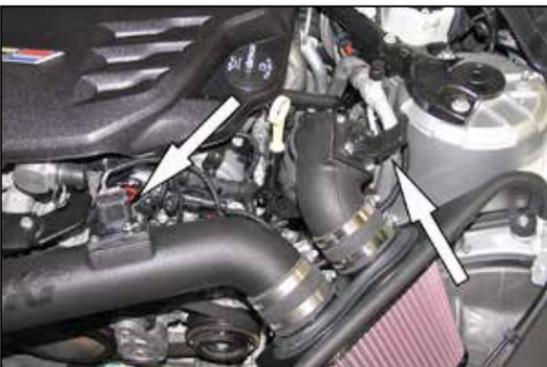
26. Reconnect the mass air sensor electrical connections.
