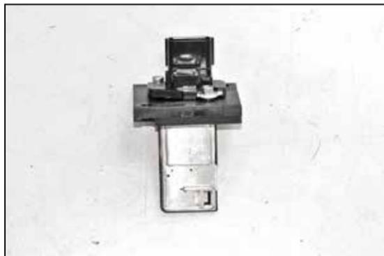
16. Install the driver's side mass air sensor into one of the K&N® adapters and secure with the provided hardware.
