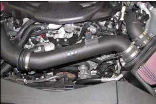
25. Install the passenger side intake tube into the coupler at the turbo inlet pipe and then into the coupler on the filter. Adjust the tubes and filter for best fit and then Secure the tubes with the provided hose clamps.
