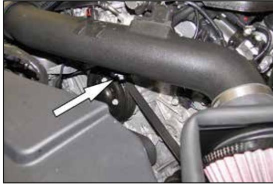
27. Connect the crank case vent hose to the quick disconnect fitting installed into the passenger side K&N® intake tube.
