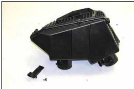
15. Remove the Drivers side mass air sensor from the factory air filter housing.
