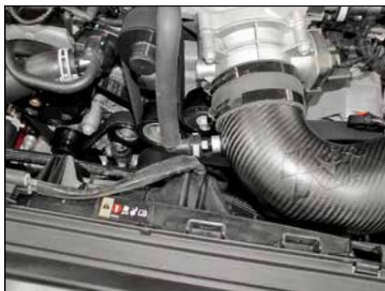
16. Connect the factory crank case vent connector into the quick disconnect fitting installed into the K&N intake tube.
