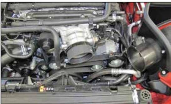
12. Install the provided coupler hose (08618) onto the throttle body and secure with the provided hose clamp.
