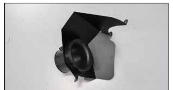
5. Install the K&N® mass air sensor housing into the Heat shield and secure with the provided hardware.
