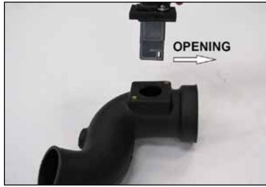
12. Install the mass air sensor assembly into the K&N® intake tube and secure with the provided hardware.
