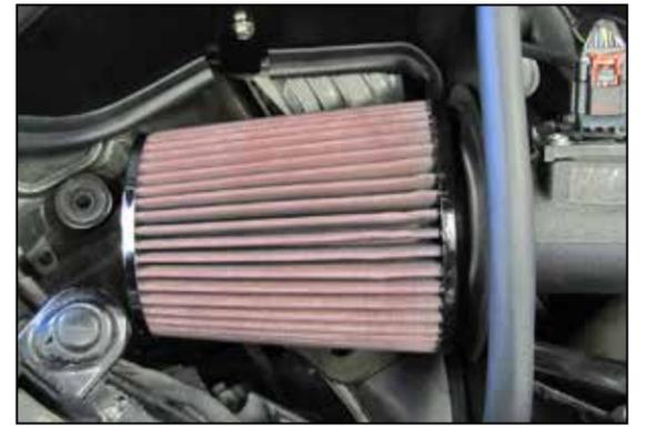
17. Install the K&N® air filter and secure with the provided hose clamp.
