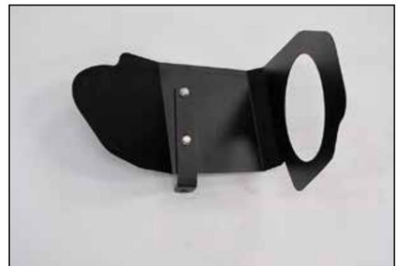
6. Install the provided "L" bracket onto the heat shield as shown using the provided hardware.
