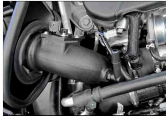
14. Install the K&N® intake tube assembly through the heat shield and then into the coupler on the turbo. Adjust the tube and heat shield for best fit and then secure the hose clamp and heat shield bolt.
