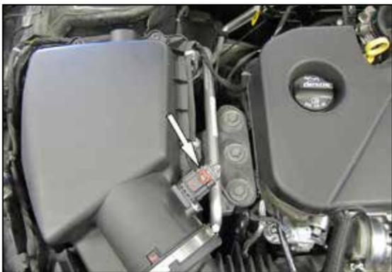
2. Release the red locking tab and then disconnect the mass air sensor electrical connection. Unhook the wiring harness from the air filter housing and set to the side.
