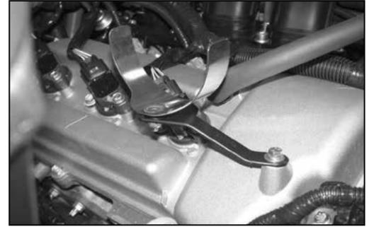
19. Install the tube mounting bracket assembly onto the valve cover with the provided hardware as shown.
