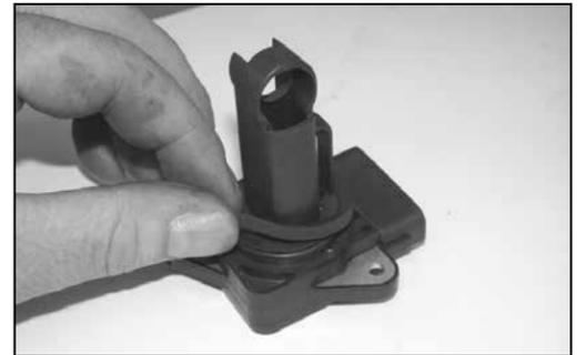
22. Apply the gasket to the mass air sensor, sticky side down as shown.
