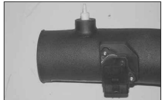
24. Install the vent fitting into the K&N® intake tube as shown.
