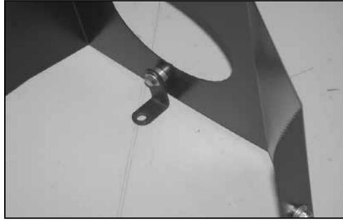
13. Install the small heat shield mounting bracket (070812) with the provided spacer onto the heat shield as shown.
