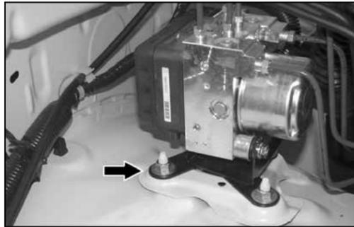
15. Remove the ABS pump mounting nut shown.
