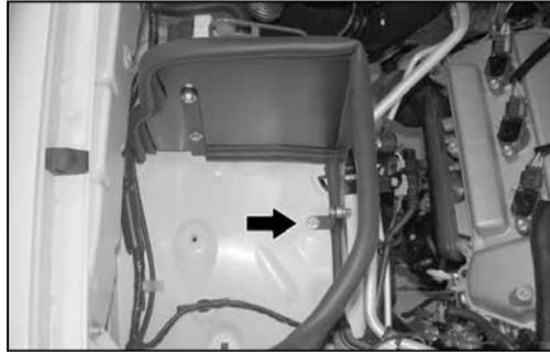
16. Install the heat shield onto the vehicle and secure with the provided hardware and the nut removed in step #15.
