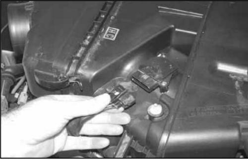
7. Disconnect the two mass air wire harness retaining clips from the air box, then disconnect the mass air sensor electrical connection.
