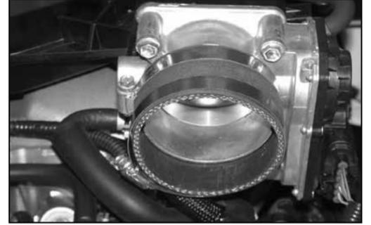
20. Install the silicone hose (08434) onto the throttle body with the provided hose clamps as shown.
