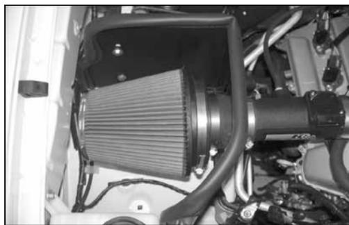
32. Install the K&N® air filter onto the intake tube as shown.
