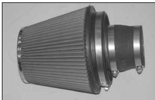
31. Install the provided silicone hose (08724) onto the air filter assembly and secure with the provided hose clamp as shown.
