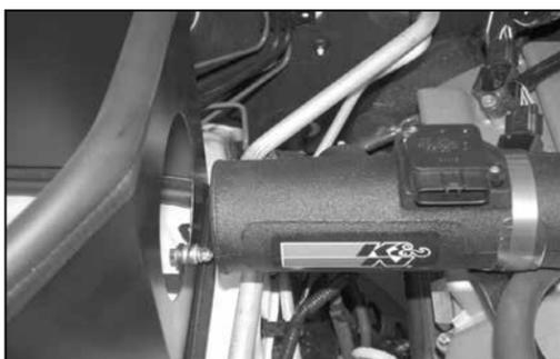
27. Secure the K&N® intake tube to the saddle bracket with the provided hose clamps. Also tighten the hose clamp attached to the throttle body.
