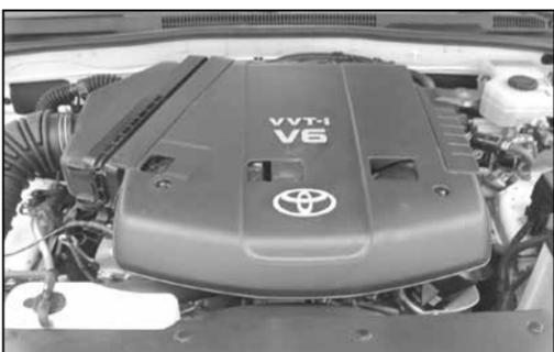
2. Loosen the two nuts that secure the engine cover, then remove the engine cover.
