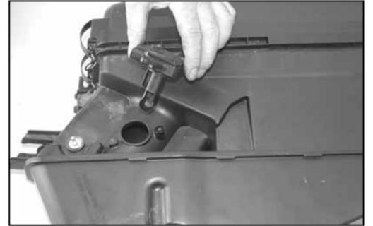
21. Remove the two screws that secure the mass air sensor to the air box assembly, then remove the mass air sensor as shown.
