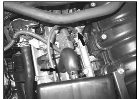
5. Disconnect the fuel pressure regulator hose from the fuel pressure regulator. Disconnect the crank case vent hose from the valve cover.
