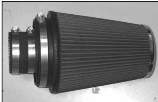
31. Install silicone hose (#08630) onto the air filter adapter and secure with the provided hose clamp.
