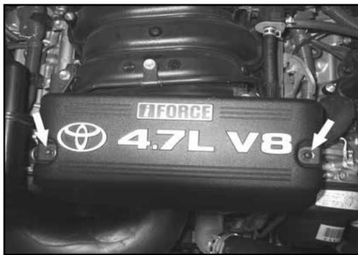
3. Remove the two factory nuts that retain the engine cover. Remove the engine cover.
