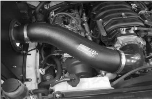
27. Install the K&N® intake tube into the silicone hose at the throttle body and align with the tube mounting bracket installed in step #11. Secure the intake tube with the provided hose clamps.
