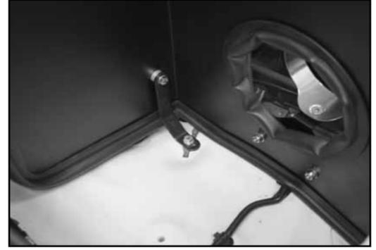
18. Set the heat shield into position on the inner fender. Secure the "C" bracket to the ground strap location.
