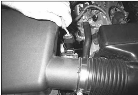
2. Disconnect the mass air sensor electrical connection, then unclip the mass air sensor wiring from the air box.
