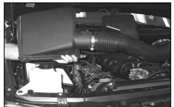
6. Release the four upper air box clam shell clamps, then remove the upper air box and intake tube assembly.
