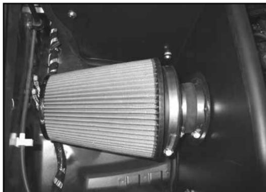
32. Install the K&N air filter assembly onto the K&N® intake tube and secure with the provided hose clamp as shown.
