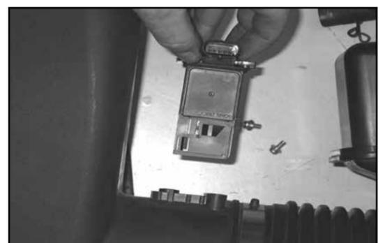
23. Remove the two factory screws that secure the mass air sensor, then remove the mass air sensor from the stock intake tube.
