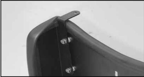
9. Install the small "L" bracket (#070742) onto the inner fender, behind the hood support. Secure with the provided hardware as shown.
