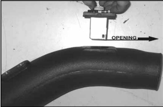
25. Install the mass air sensor assembly into the K&N® intake tube and secure with the provided hardware.
