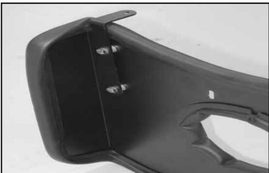
12. Install the long "L" bracket (#070902) onto the heat shield with the provided hardware as shown.
