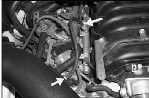
29. Install the provided fuel pressure hose onto the fuel pressure regulator, then connect the open end to the NPT fitting installed into the K&N® intake tube as shown.
