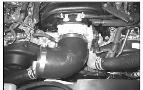
21. Install silicone hose (#084086) onto the throttle body and secure with the provided hose clamp.
