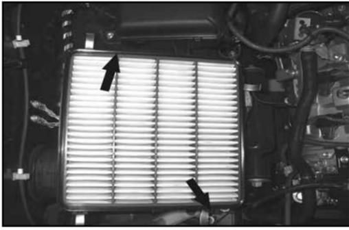
7. Remove the two factory bolts that secure the lower air box to the inner fender.
