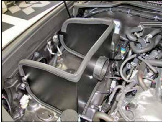
13. Set the heat shield into the engine compartment and secure with the provided hardware.
