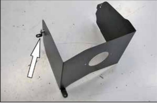
8. Install the heat shield mounting bracket (070066) onto the heat shield using the provided spacer and hardware.
