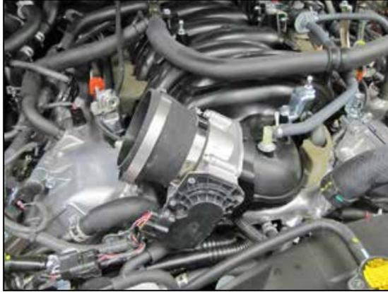
14. Install the coupler hose (08050) onto the throttle body and secure with the provided hose clamp.
