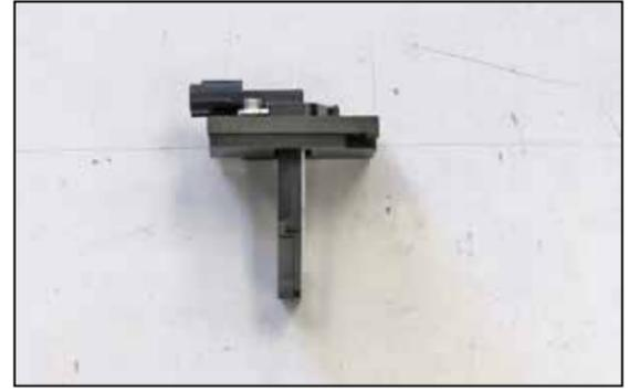
18. Install the mass air sensor assembly into the K&N® mass air sensor adapter as shown using the provided hardware.
