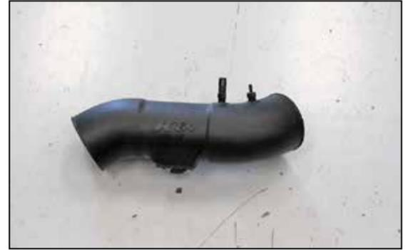
20. Install the provided NPT vent fittings into the K&N® intake tube as shown.
