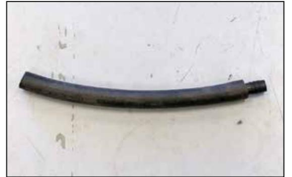
21. Install the hose mender into the provided crank case vent hose as shown.
