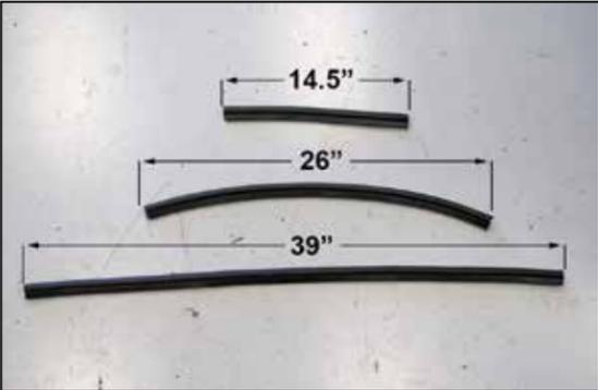
9. Cut the provided edge trim into three sections. One section will be 39" long, one section will be 26" long and the final section will be 14.5" long.
