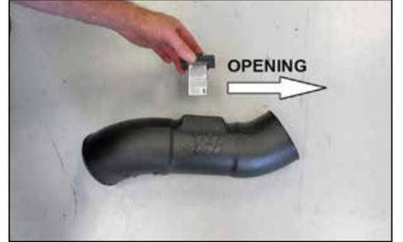
19. Install the mass air sensor assembly into the K&N® intake tube and secure with the provided hardware.
