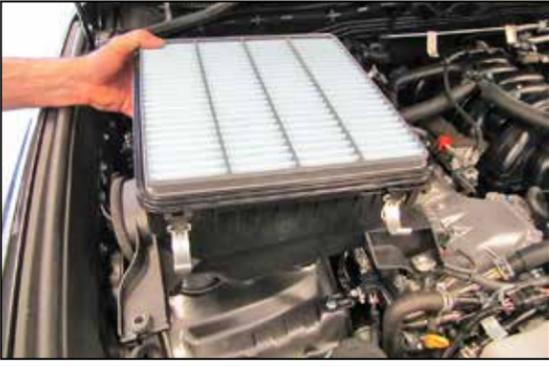
7. Loosen the three bolts securing the lower air box and then remove the lower air box from the vehicle.
