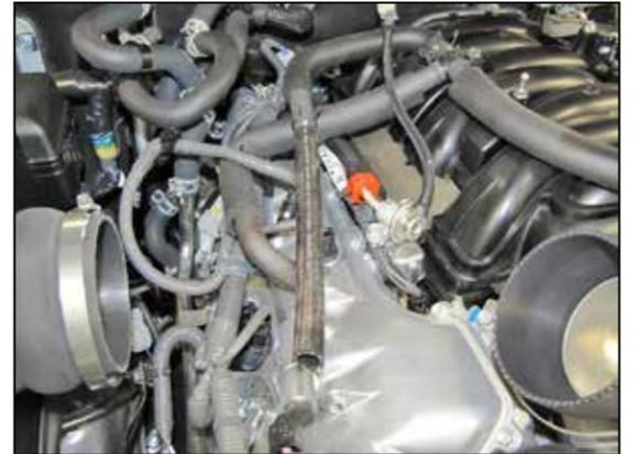
22. Install the crank case vent hose assembly into the factory crank case vent hose as shown.
