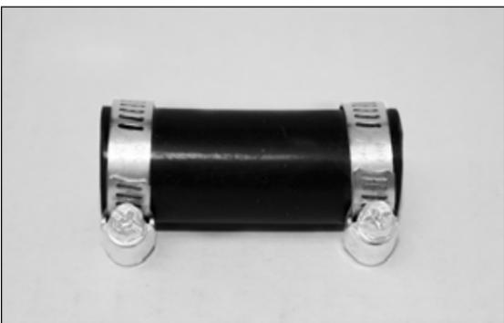
15. **2005-06 Model Year Vehicles ONLY:** On '05-'06 models, place hose clamps on each side of the silicone hose (08692), as shown.
