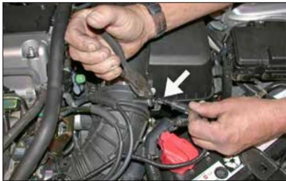
4. Using a pair of pliers, depress the hose clamp and remove the air temperature sensor from the stock intake tube as shown.
