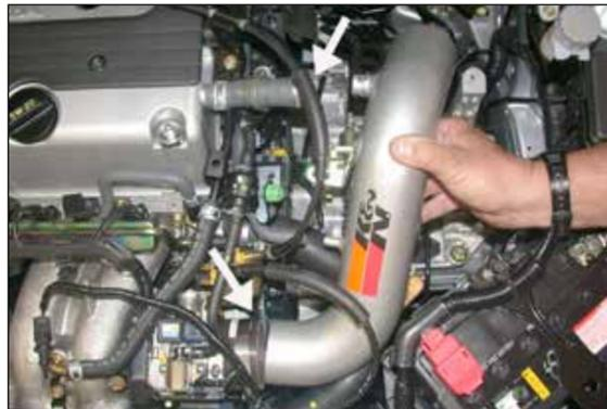
18. Install the second hose clamp onto the silicone hose, then, slide the K&N® intake tube into the silicone hose as shown. Line up the intake tube bracket with the original air cleaner mounting point.
