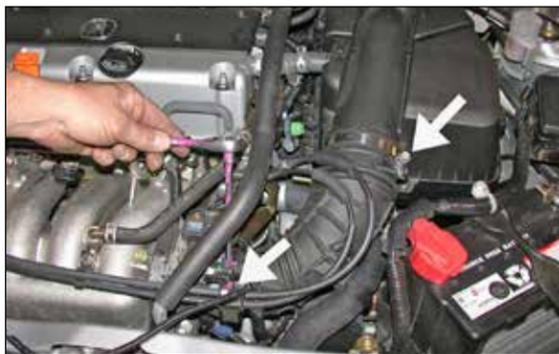
5. Loosen the two hose clamps at the throttle body and at the air cleaner assembly as shown.
