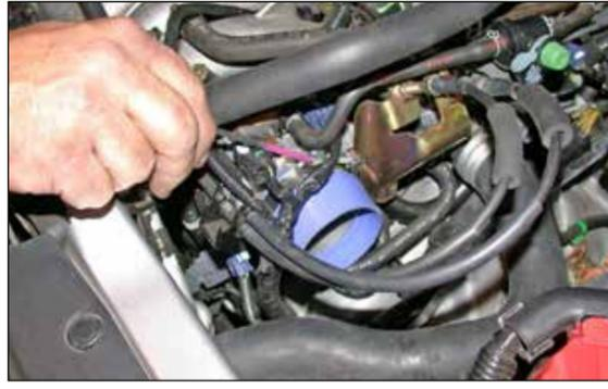
16. Install the silicone hose and hose clamp onto the throttle body as shown.
