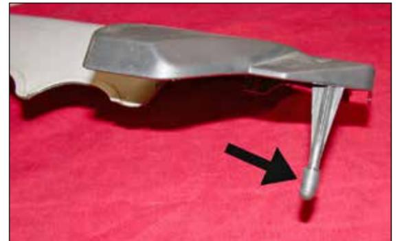
25. Install the rubber cap plug onto the stand off on the engine cover as shown.
