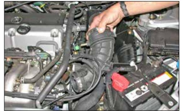
9. Pull the stock intake tube off of the throttle body, then remove the stock intake tube as shown.
