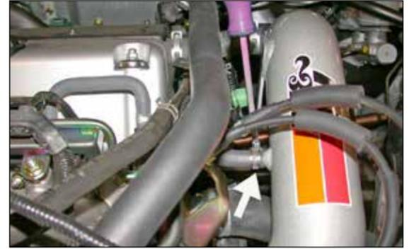
22. Reconnect the idle air bypass control thermal valve vent hose to the vent on the K&N® intake tube and secure with the provided hose clamp as shown.
