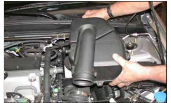
8. Loosen the 5 bolts and pull upwards to remove the upper air cleaner assembly as shown.
