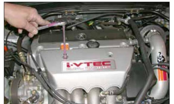
26. Reinstall the engine cover as shown.
