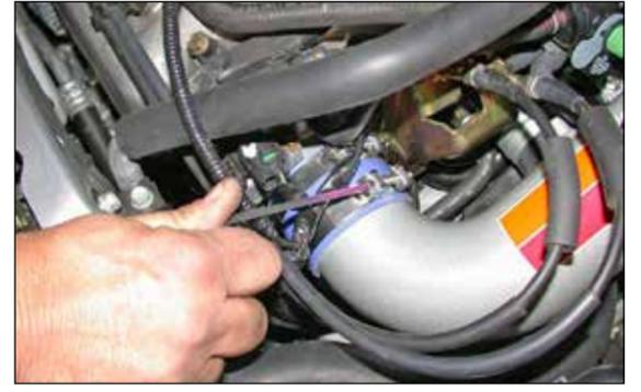
21. Using a flat blade screwdriver, tighten the hose clamp on the silicone hose as shown.
