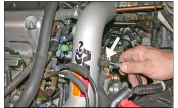
23. Push the air temperature sensor into the grommet on the K&N® intake tube as shown.
