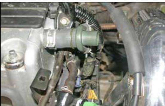
14. **2005-06 Model Year Vehicles ONLY:** On '05-'06 models, remove the stock crank case vent hose as shown.
