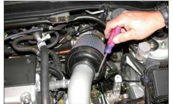
24. Install the K&N® air filter onto the K&N® intake tube and secure with the provided hose clamp as shown.
