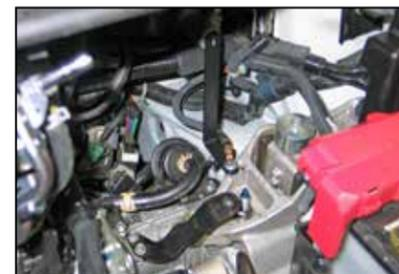
11. Install the heat shield mounting bracket (083112) onto the ground strap location from step #10. Be sure to secure the ground strap on top of the installed bracket.
