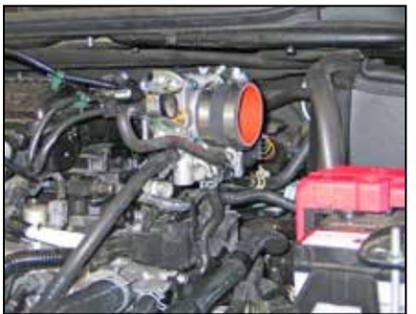
16. Install the provided silicone hose (08284) onto the throttle body and secure with the provided hose clamp.
