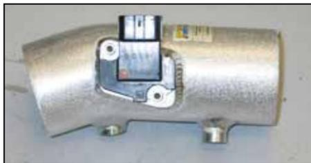
18. Install the mass air sensor into the K&N intake tube and secure with the provided hardware.
