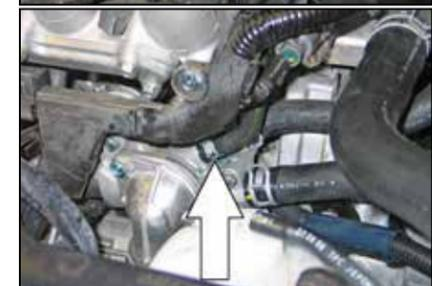
14. **Be sure the engine is cool and the cooling system is not under pressure.** Loosen the hose clamps and remove the coolant bypass hose from the throttle body and thermostat housing. Be sure to capture any lost coolant in an appropriate container.
