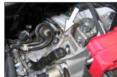
10. Remove the bolt which secures the ground strap to the transmission mount.
