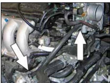
15. Install the provided coolant bypass hose and secure with the provided hose clamps. Be sure to replace any lost coolant.
