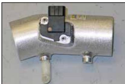
19. Install the provided 90° npt fitting into the K&N intake tube as shown.
