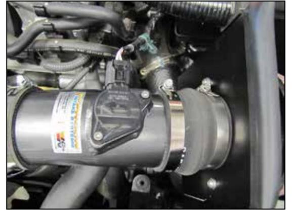
16. Reconnect the mass air sensor electrical connection.
