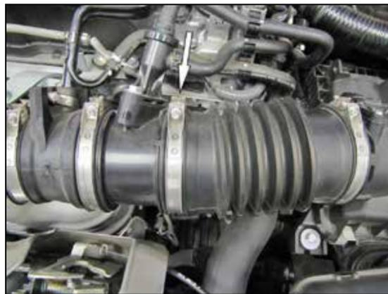
3. Loosen the hose clamp that secures the intake hose to the turbo inlet tube.
