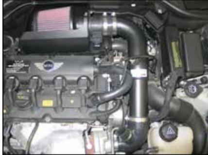
15. Install the K&N® intake tube into the silicone hoses on the turbo inlet and mass air sensor and then secure with the provided hose clamp.
