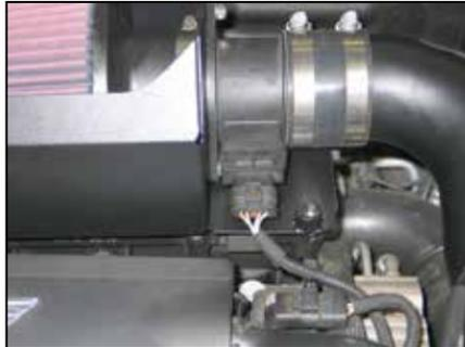
17. Reconnect the mass air sensors electrical connection.
