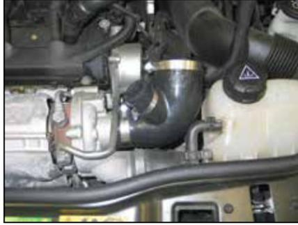
14. Install the silicone hose (08484) onto the turbo inlet and secure with the provided hose clamp.
