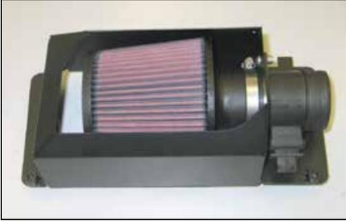
10. Install the K&N® air filter onto the mass air sensor inside the heat shield and secure with the provided hose clamp.
