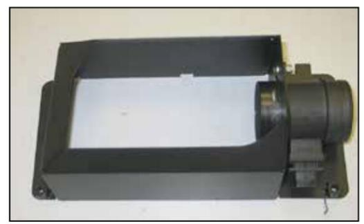
9. Install the mass air sensor into the heat shield and secure with the provided hardware. **NOTE: Be sure to install the button head bolts from the inside of the heat shield out.**
