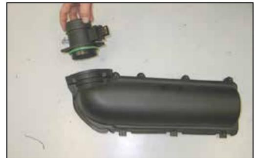
7. Remove the two screws which secure the mass air sensor to the upper airbox and then remove the mass air sensor from the upper airbox.
