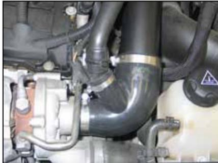
16. Install the crankcase vent hose into the silicone hose at the turbo inlet and secure with the provided hose clamp.
