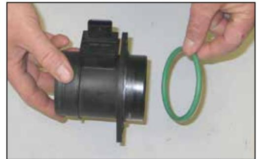
8. Remove the mass air sensor from the airbox, and then remove the "O" ring gasket from the mass air sensor.
