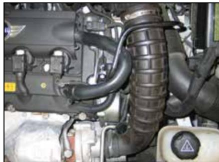
4. Loosen the two hose clamps which secure the intake tube to the turbo inlet and airbox.
