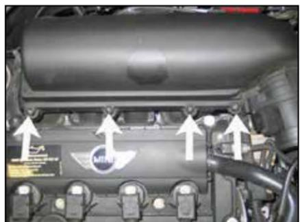
6. Loosen the four screws which secure the upper airbox to the lower airbox, then remove the upper airbox and air filter from the vehicle.
