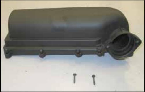
12. Remove two of the upper airbox mounting screws from the upper airbox.
