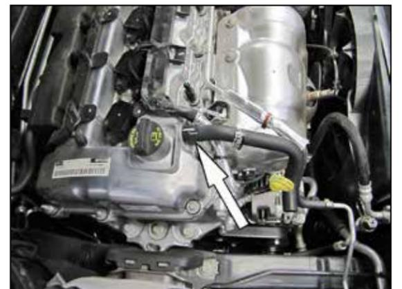
8. Remove the crank case vent hose from the valve cover port.
