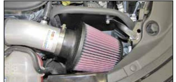
23. Install the K&N® air filter and secure with the provided hose clamp.
