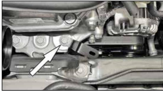
17. Install the tube mounting bracket #064301 onto the engine mount and secure with the factory bolt from the previous step.
