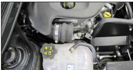
19. Install the provided hump hose #08696 onto the plenum inlet and secure with the provided hose clamp.
