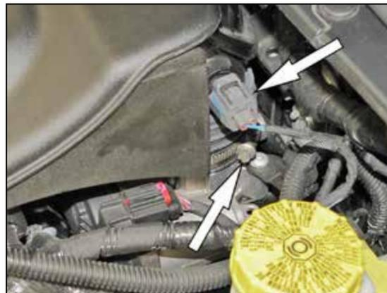
6. Disconnect the inlet air temperature sensor electrical connection and then loosen the hose clamp securing the intake plenum to the throttle body.
