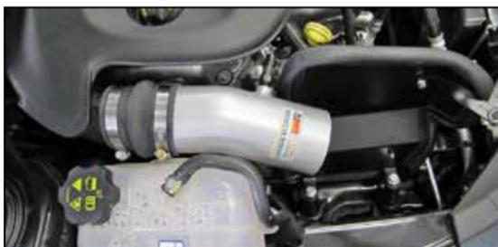
21. Install the K&N® intake tube into the silicone hose and align with the mounting bracket previously installed. Secure the tube with the provided hardware and hose clamp.
