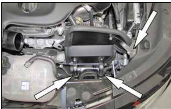
18. Install the heat shield mounts into the factory mounting grommets and then secure mounting bracket to the core support with the factory air box mounting bolt.
