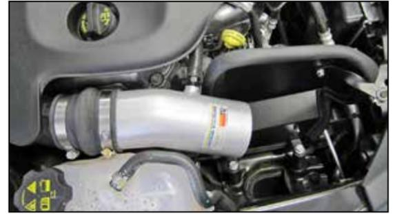
22. Connect the crank case vent hose to the fitting installed into the K&N® intake tube.
