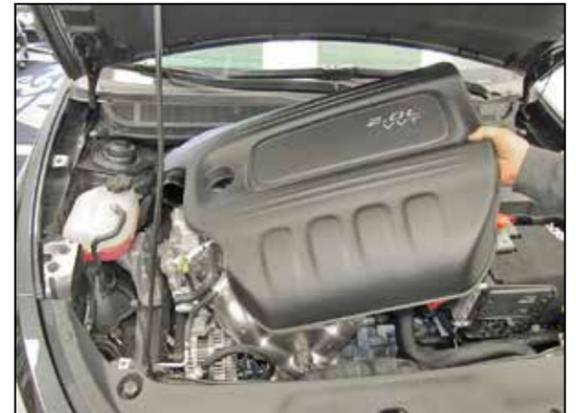
7. Lift up and remove the intake plenum from the vehicle.
