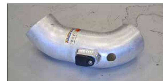
17A. On vehicles equipped with the round style sensor, mark the intake tube as shown 1.0 to 1.25" from the sensor boss. Drill a 3/4" id hole on the mark.
