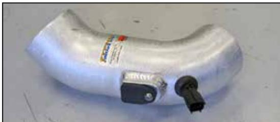
17b. Install the provided grommet into the hole drilled. Then remove the O-ring from the sensor and install the sensor into the grommet.
