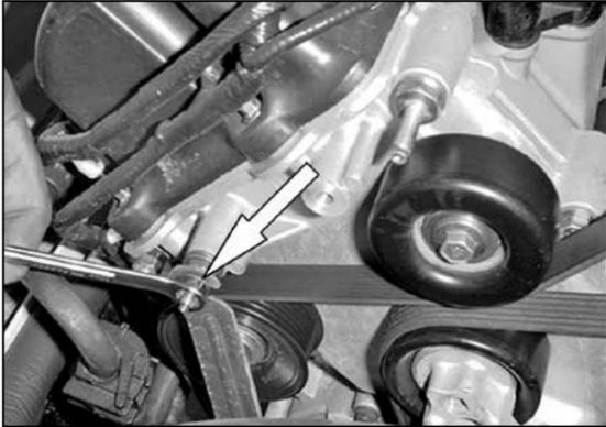
11. Loosen and remove the nut from the protruding stud on the engine.
