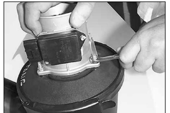
9. Loosen and remove the 4 nuts that retain the mass air sensor.
