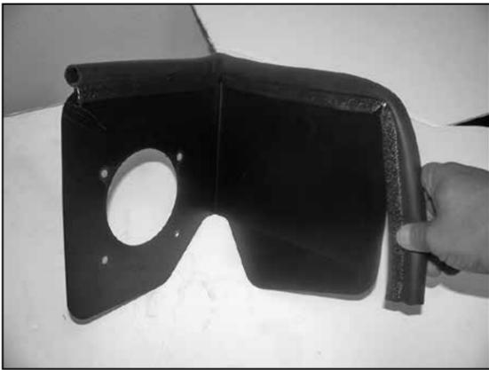
12. Install the trim seal onto the heat shield.
