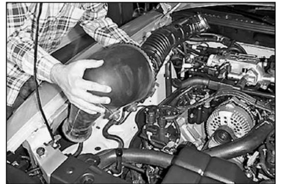
7. Remove the entire air intake assembly.
