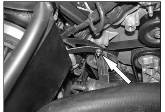
22. Slide the brackets onto the stud from step 11 and secure with the factory nut.
