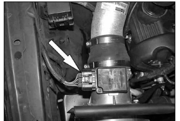
24. Reconnect mass air sensor electrical connection as shown.
