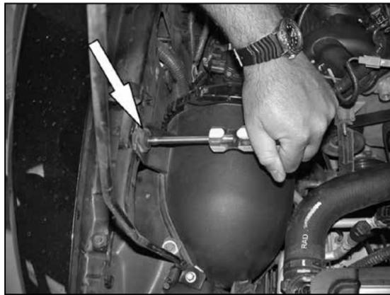
4. Loosen and remove the bolt that retains the air cleaner.
