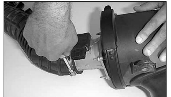
8. Loosen the hose clamp and detach the intake tube from the mass air sensor.
