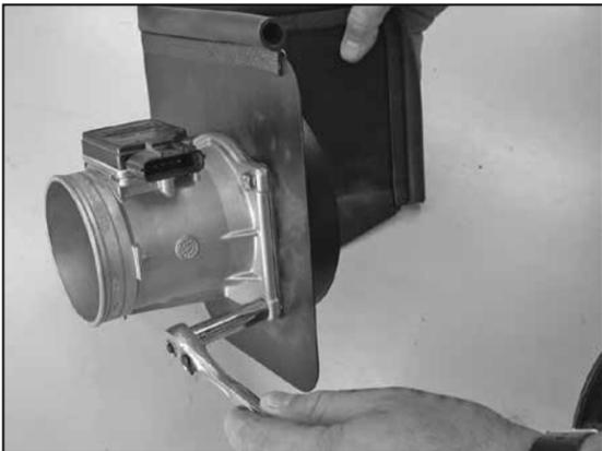
13. Assemble the mass air sensor, heat shield and adapter, using the gaskets and hardware provided as shown, but do not tighten completely at this time.
