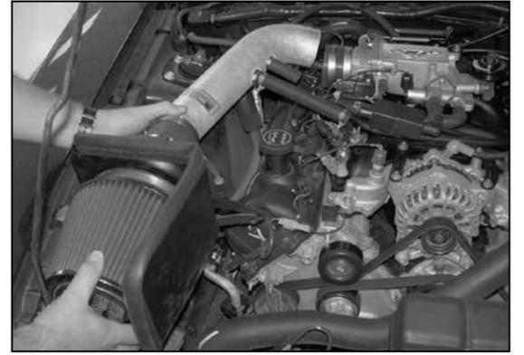
21. Install the complete K&N® intake assembly into the vehicle and slide the tube into the silicone hose on the throttle body as shown.
