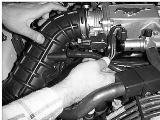
6. Detach the PCV line from the intake tube.
