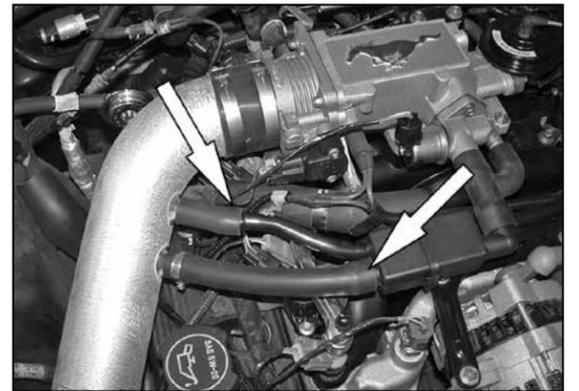
23. Reconnect the vent hoses to the K&N® intake tube as shown and tighten hose clamps.
