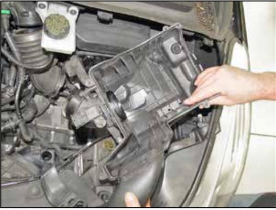
7. Lift up the lower air filter housing to dislodge it from the mounting grommets then rotate the housing up and remove it from the vehicle. Remove the factory intake tube at this time.
