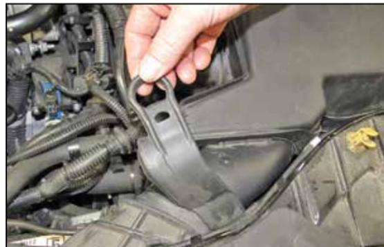
4. Release the rubber strap that secures the fresh air intake hose.
