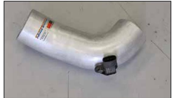
20. Install the inlet air temperature sensor into the grommet installed into the K&N® intake tube.
