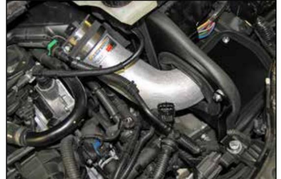
21. Install the K&N® intake tube through the heat shield and then into the coupling hose and secure with the provided hose clamp.
