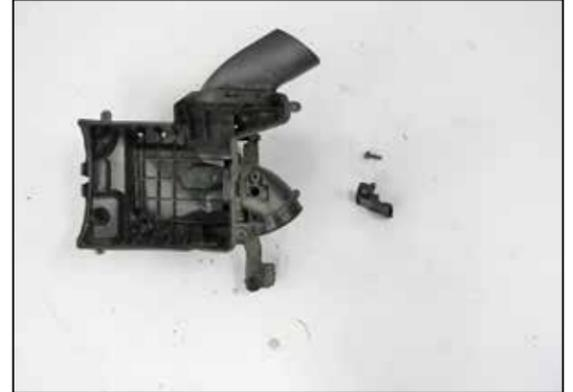
19. Remove the inlet air temperature sensor from the factory air filter housing.
