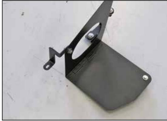
13. Install the provided bracket (064334) onto the heat shield as shown.
