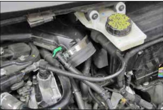
9. Install the provided coupler (08190) onto the turbo inlet tube and secure with the provided hose clamp.
