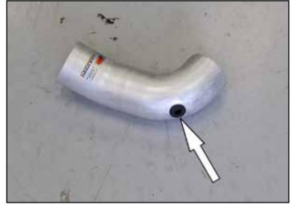
18. Install the provided grommet into the K&N® intake tube as shown.
