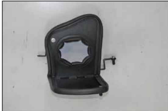
15. Install the 16" edge trim into the hole of the heat shield and install the 44" edge trim around the outside of the heat shield as shown.
