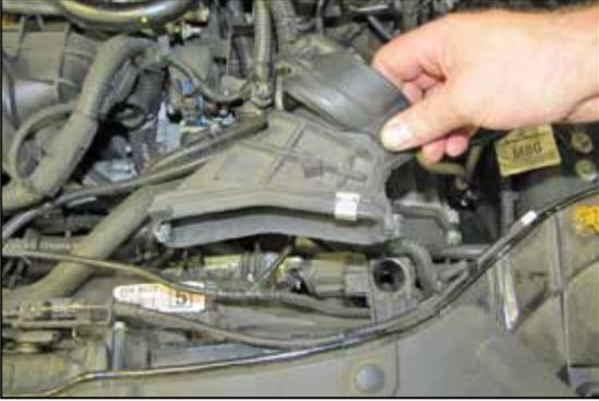
8. Remove the rubber fresh air intake duct.
