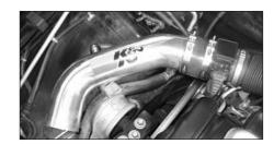
12. Align the tube and gently remove the tube. (in this way you have the bracket in the right position.)
