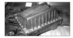
6. Remove the complete air box from the vehicle as shown.
