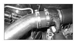
14. Refit the tube into the sleeve and firmly tighten the #44 hose clamp.
