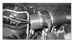
7. Fit the silicone sleeve onto the MAS using the #44 hose clamp supplied.
