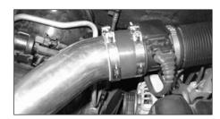
10. Fit the tube into the silicone sleeve using the #44 hosel clamp. (Do not fully tighten at this moment.) **NOTE**: Before installing, clean the inside of out with water and a towel!
