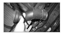
2. Remove the air box feed pipe from between the air box and intake snorkel as shown.
