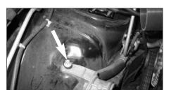
8. Remove the bolt of the engine support bracket as shown.
