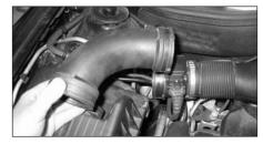
3. Unclip and remove the intake hose from between the air box and the mass air sensor (MAS).
