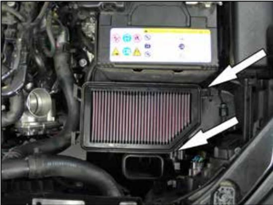
9. Remove the two bolts securing the lower air box to the vehicle and then remove the lower air box from the vehicle.
