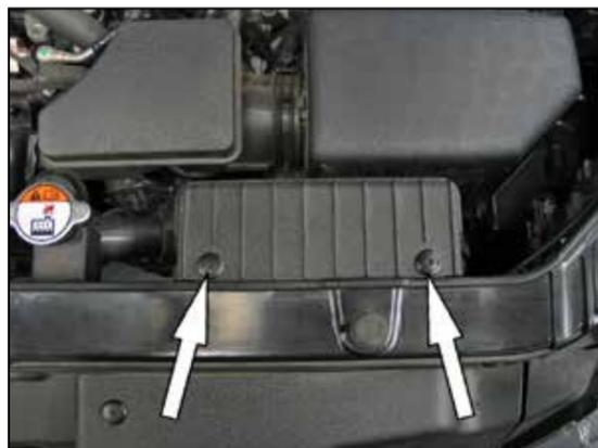
4. Remove the two plastic screws securing the fresh air intake scoop and then remove the clips.
