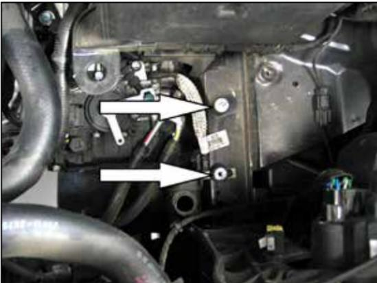
11. Install the two 1" rubber mounted studs as shown. One will screw into the threaded hole vacated by the ground strap bolt in step #10 and the other will thread onto the unoccupied stud on the frame rail.
