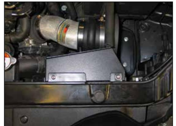
21. Install the K&N® fresh air intake scoop and secure to the heat shield and core support with the provided hardware.
