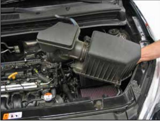
8. Remove the upper air box from the vehicle.
