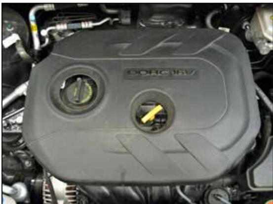
2. Pull up the engine cover and remove it from the engine.
