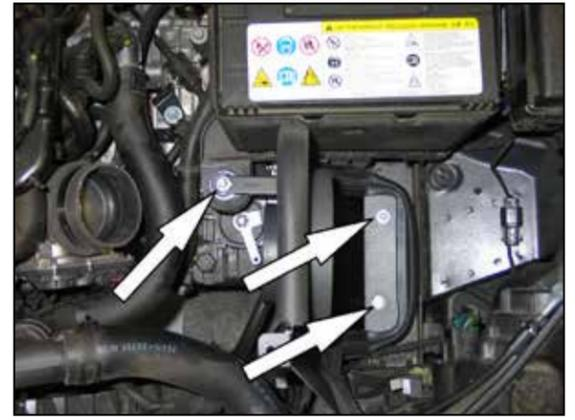
17. Install the heat shield onto the rubber mounted studs and secure with the provided hardware.
