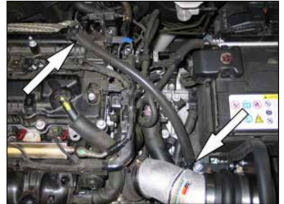
20. Install the provided crank case vent hose onto the 90° vent fitting and valve cover port as shown.
