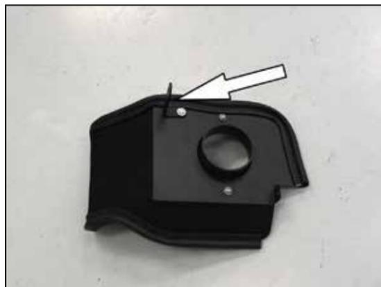
16. Install the provided "L" bracket (07093) onto the heat shield as shown using the provided hardware.
