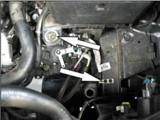
10. Remove the air box mounting grommet shown, and then remove the inner most ground strap bolt shown.
