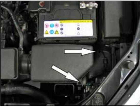
7. Unlatch the two upper air box retaining clips.
