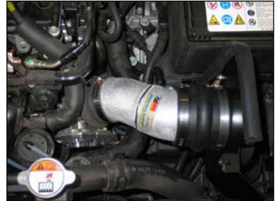
19. Install the provided hump hose (5-576) onto the filter adapter and secure with the provided hose clamp. Then install the K&N® intake tube and secure with the provided hose clamps.
