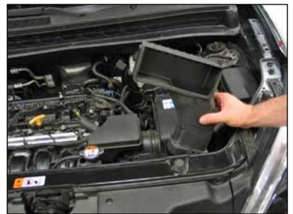
5. Lift up the fresh air scoop and remove it from the vehicle.
