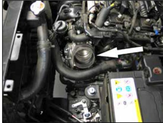
13. Install the provided hump hose (08421) onto the throttle body and secure with the provided hose clamp.
