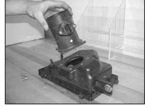
10. Loosen and remove the four hex bolts to remove the mass air sensor from the stock air cleaner lid as shown.
