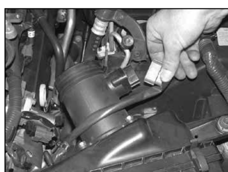
6. Disconnect the mass air sensor electrical connection as shown.
