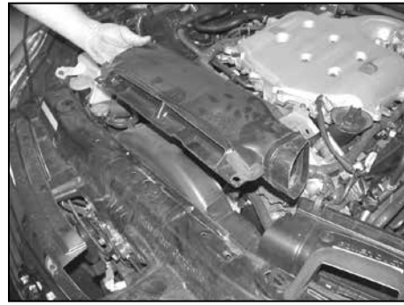
8. Disengage the two plastic rivets, then, remove the stock air inlet duct as shown.
