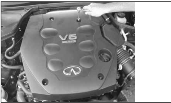
2. Remove the engine cover as shown.
