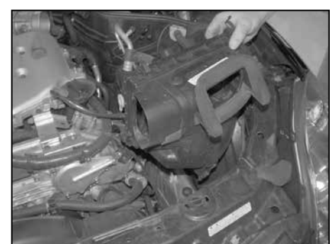
9. Pull firmly upwards to release the air cleaner base from the factory grommets, then remove the air cleaner base as shown.
