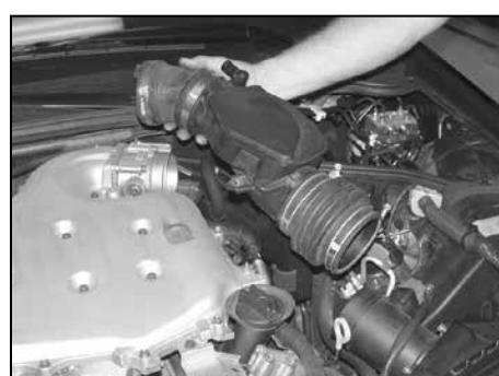
5. Remove the stock intake tube as shown.
