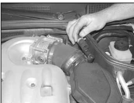
3. Disconnect the crankcase vent hose as shown.
