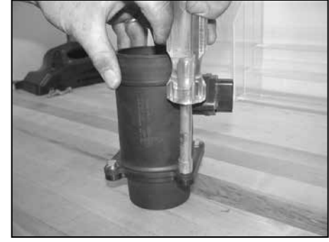
11. Assemble the provided mass air adapter onto the stock mass air sensor using the provided hardware as shown.
