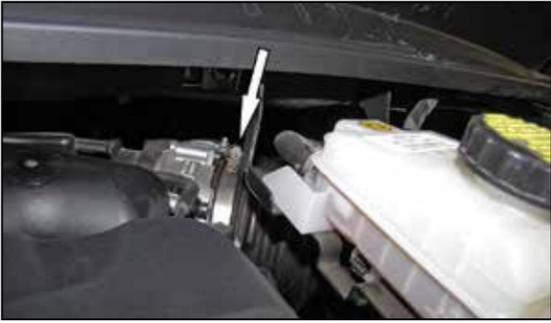
7. Loosen the hose clamp securing the factory intake tube to the throttle body and then remove it from the vehicle.
