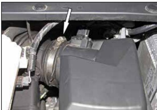
4. Loosen the hose clamp that secures the factory intake tube to the air filter housing.
