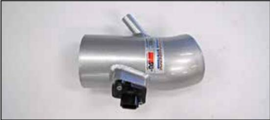
8. Remove the mass air sensor from the factory air box and then install it into the K&N intake tube and secure with the provided hardware.
