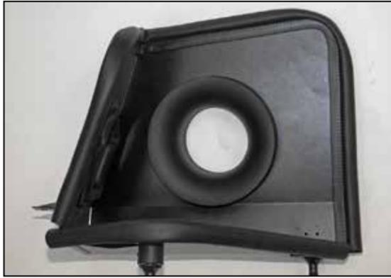
13. Install the K&N filter adapter into the heat shield and secure with the provided hardware.
