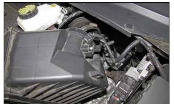
6. Partially remove the air filter housing to access the transmission vent line, mass air sensor and wiring harness, disconnect the mass air sensor and wiring harness and trans mission vent line and then remove the air filter housing from the vehicle.
