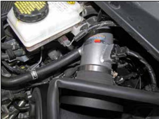
17. Install the hose mender into the factory crankcase vent hose and secure with the factory spring clamp then connect the open end of the hose to the port on the K&N intake tube.
