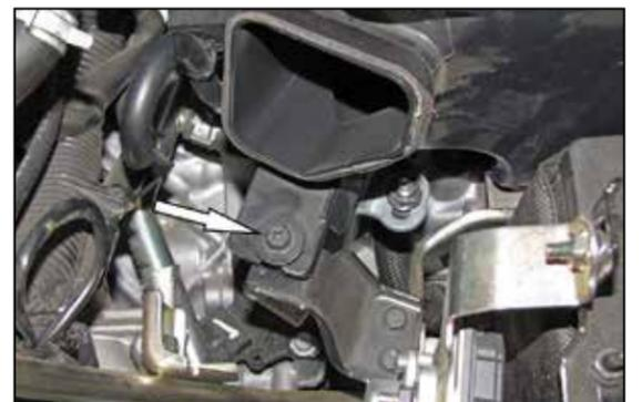
5. Remove the bolt which secures the air filter housing to the mount.
