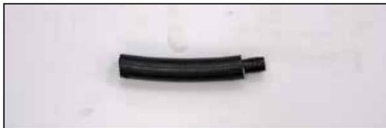
16. Install the provided hose mender into the provided crankcase vent hose as shown.
