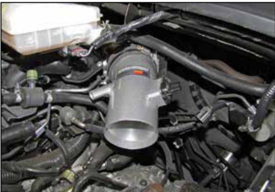
9. Install coupler hose (08690) onto the throttle body and secure with the provided hose clamp. Then install the K&N intake tube into the coupling hose as shown.
