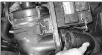
5. Disconnect the 2 air box feed pipes from the air box as shown.
