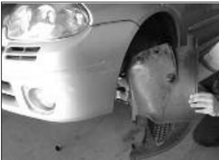
24. Re-install the wheel arch liner using its original hardware. Now re-install wheel to the vehicle. Re-install the front wheel and torque it up to factory specifications!
