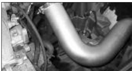
17. Feed the intake tube into the wheel arch area. Locate the vibration mount into the hole in the inner wing, secure with an M6 nut and washer supplied. Don't fully tighten yet!
