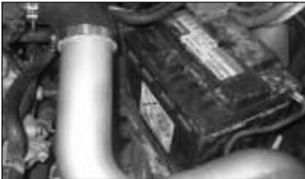
22. Re-install the battery to the vehicle and reconnect the battery terminals (positive terminal first).
