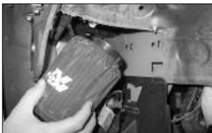
20. Fit the filter on to the intake pipe using the #44 hose clamp supplied. Align the complete intake tube assembly for maximum clearance. Now firmly tighten all hose clamps and hardware.
