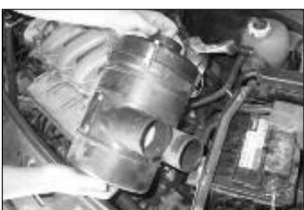
6. Unclip and remove the complete air box assembly from the vehicle.
