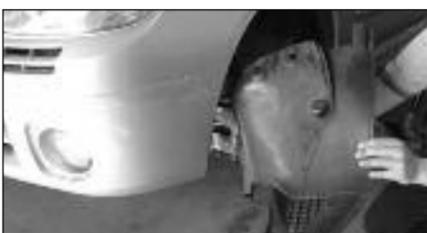
11. Remove the L/H wheel arch liner.
