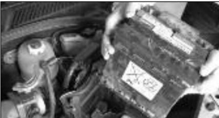
8. Disconnect first the negative, then the positive cable from the battery & remove the battery from the vehicle.
