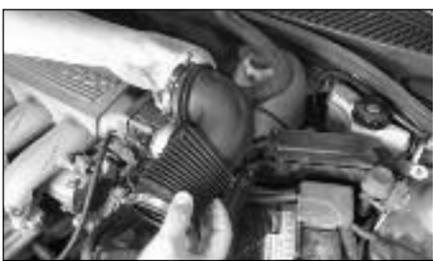
4. Unclip & remove the complete intake hose assembly.
