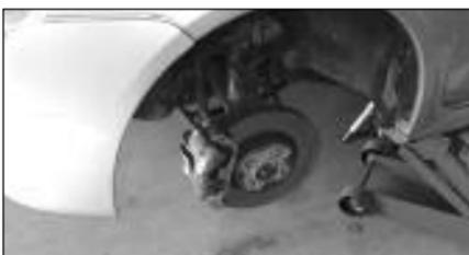
10. Taking the necessary safety precautions raise the front of the vehicle and support it with axle stands. Now remove the L/H front wheel as shown.
