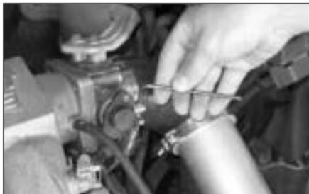
18. Fit the silicone hose on to the throttle housing using the #44 hose clamp supplied. Don't fully tighten yet!
