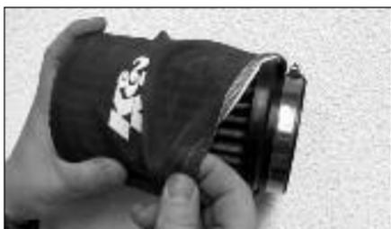
19. Fit the drycharger on to the filtercharger as shown. **NOTE:** The Drycharger's water repellent properties will last up to two years. See the parts list to order Drycharger if necessary.
