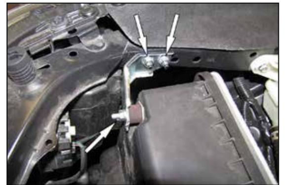
5. Remove the three nuts that secure the air filter housing to the inner fender and then remove the bracket from the vehicle.
