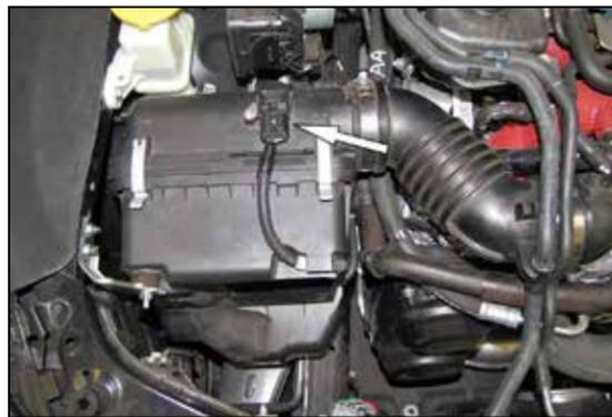
3. Disconnect the mass air sensor electrical connection and unclip the wiring harness from the air filter housing.
