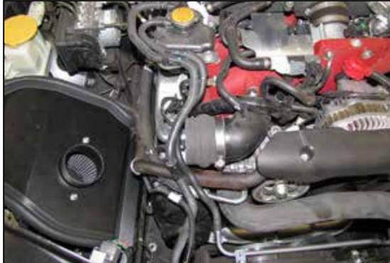
13. Install the provided hump coupler (08185) onto the turbo inlet tube. Set the heat shield assembly into position on the inner fender but do not secure.
