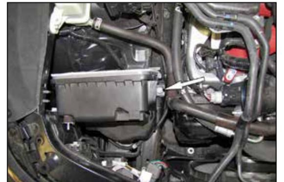
6. Remove the bolt that secures the dirty side air filter housing to the frame rail and then remove the air filter housing from the vehicle.
