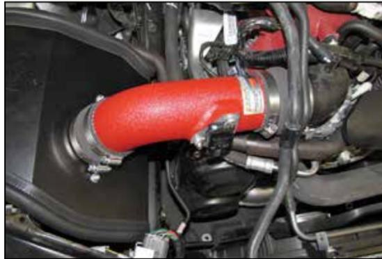
14. Install the K&N® intake tube into the coupler at the turbo inlet tube and align with the filter adapter, slide the coupler onto the filter adapter, adjust the tube for best fit and secure with the hose clamps. Secure the heat shield with the provided hardware.
