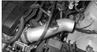
30. Slide the Typhoon tube into the silicone step hose, but don't fully tighten the hose clamp yet!
