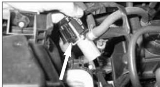
7. Push back the indicated clip and remove the PWM vacuum switching valve from the air box lid.
