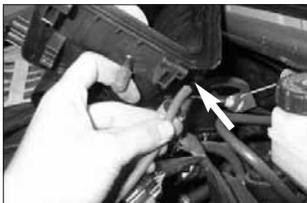
6. Unclip the air box lid, then tilt upwards and remove the vacuum hose as shown.
