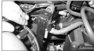
32. Slide the PWM vacuum switching valve onto the "L" bracket as shown.
