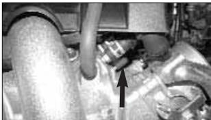
22a. **2002-2004 models:** Install the small rubber cap plug onto the vent on the manifold as shown.
