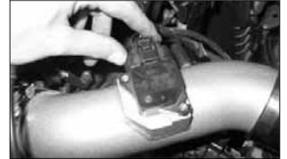
35b. Re-connect the mass air sensor electrical connection as shown.
