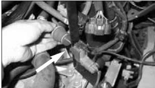
24. Secure the vacuum switching valve or relay unit to the "L" bracket using the screw removed in step 4.
