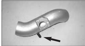
26. Fit the large rubber cap plug over the vent in the Typhoon intake tube as shown.
