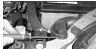
15. Remove the push clip that secures the air inlet duct to the radiator core support as shown.
