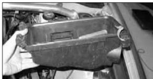
11. Remove the air box base as shown. **NOTE: K&N recommends that customers do not discard factory air intake.**
