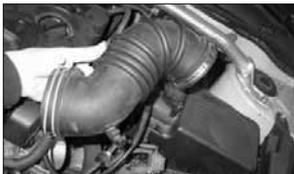
5. Loosen the hose clamps at the throttle body and at the air box, then release the vacuum hose from the stock intake tube and remove the stock intake tube as shown.
