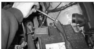
12. Loosen the battery hold down bracket as shown.
