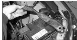
14. Remove the bolt that secures the battery hold down bracket to the vehicle, then, remove the battery hold down bracket as shown.
