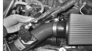
35a. **UK models:** It will be necessary to increase the length of the MAS plug wiring harness. Undo the insulation tape where the MAS harness enters the main harness & carefully pull the harness out to increase the length. Re-apply insulation tape to the harness.
