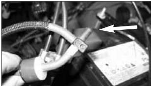
21b. **2005-later & compressor models:** Remove the vacuum hose from the vacuum connector and replace it with the small rubber cap plug as shown.
