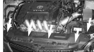
37. Reinstall the radiator core cover using the original 4 clips and 2 bolts as shown.
