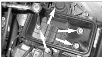
9. Loosen and remove the three bolts that secure the air box base to the vehicle as shown. Also disconnect the indicated vacuum hose from the butterfly valve.
