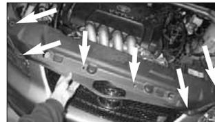
13. Loosen the 4 clips and the 2 bolts, then, remove the radiator core cover as shown.
