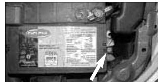
16. Loosen and remove the bolt that secures the air inlet duct to the inner fender as shown.
