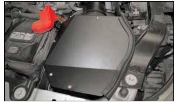
36. Install the heat shield lid onto the heat shield and secure with the provided hardware.
