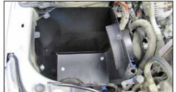
23. Set the heat shield assembly into position and secure with the factory mounting hardware from step #12.
