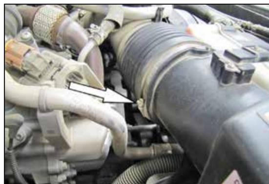
3. Loosen the hose clamp which secures the intake tube to the upper air box.
