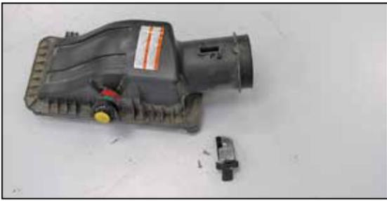
25. Remove the two screws securing the mass air sensor into the factory air box and then remove the sensor from the air box.
