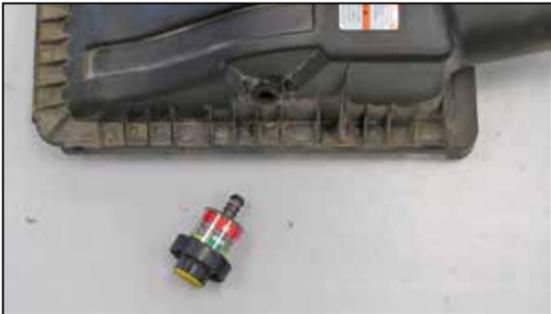
27. Remove the Filter minder from the factory air box housing.
