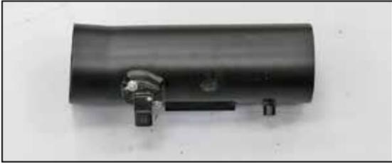
26. Install the mass air sensor assembly into the K&N® intake tube as shown and secure with the provided hardware.
