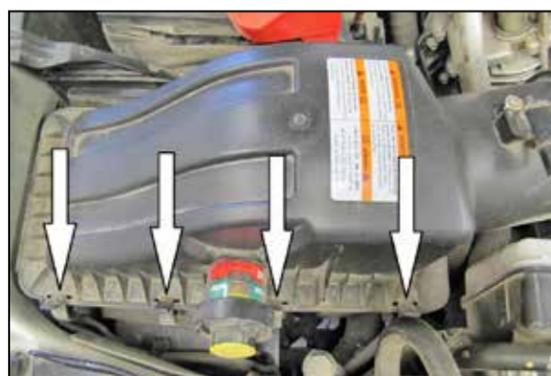
4. Release the four upper air box retaining clips.
