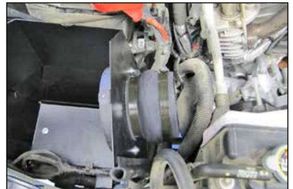
24. Install the silicone hump hose (08418) onto the filter adapter and secure with the provided hose clamp.
