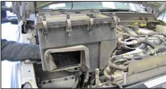
10. Remove the lower air box from the vehicle.
