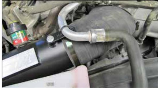
32. Secure the coolant pipe with the provided bracket (083166), mounting tie wrap and hardware to threaded stand-off on the K&N® intake tube.
