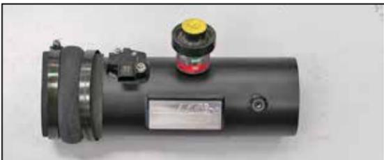
29. Install the provided silicone hump hose (08418) onto the K&N® intake tube.
