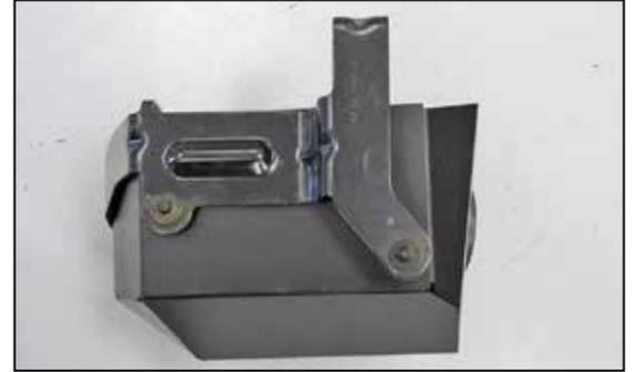
21. Install the factory air box mounting bracket onto the heat shield as shown so that the mount stand-offs installed in step #20 snap into the factory mounting grommets.
