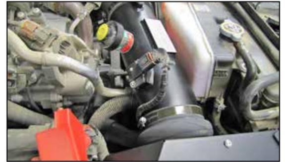
37. Reconnect the mass air sensor electrical connection.
