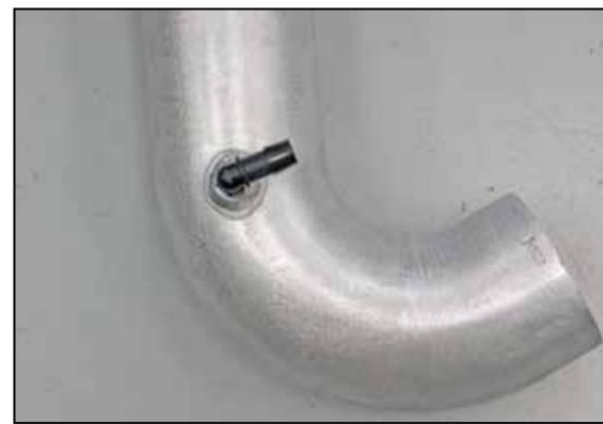
20. Install the 90° npt fitting into the K&N® intake tube as shown.
