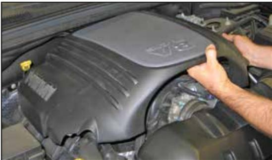
2. Lift up the engine cover to dislodge it from the mounting grommets and remove it from the vehicle.
