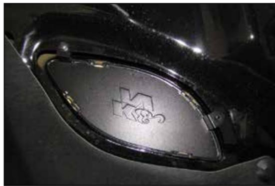
26. Place the provided block off into position and reinstall the factory screws.
