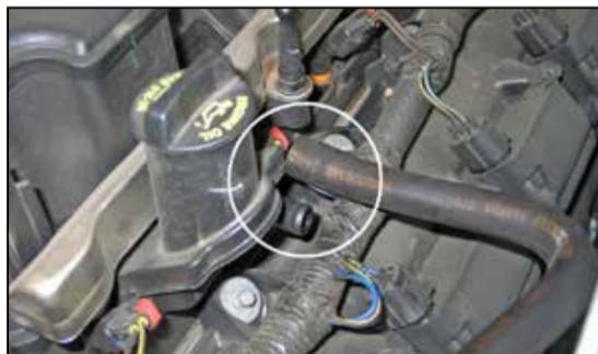
5. Disconnect the crank case vent hose from the valve cover port.
