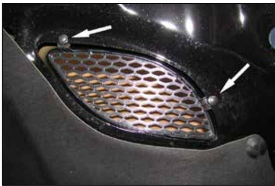
25. Some Dodge Durango models may be equipped with heat extractor vents in the hood. During inclement weather or driving in wet conditions, K&N® recommends installing the provided heat extractor block off plate. Remove the two screws that secure the factory grid in position.
