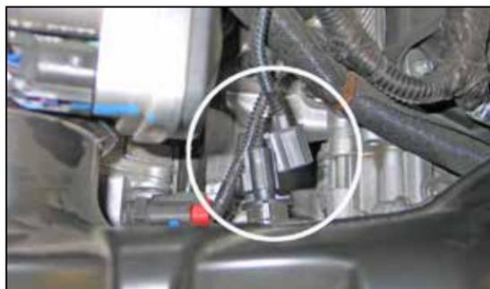
4. Disconnect the inlet air temperature air sensor electrical connection.
