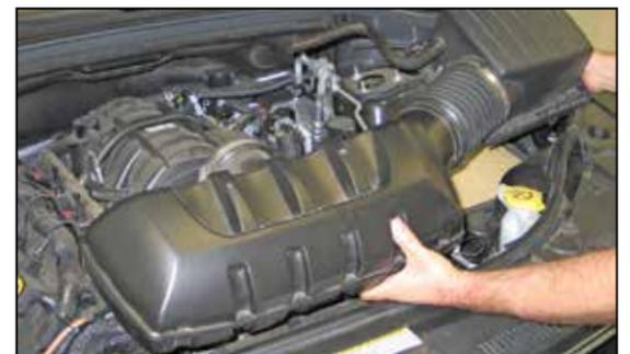
7. Remove the upper air box and intake tube assembly.
