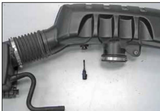
18. Release the locking tab and then remove the inlet air temperature sensor from the factory intake tube by twisting counter clockwise.
