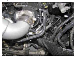
23. Reconnect the inlet air temperature sensor electrical connection.
