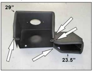
9. Install the two sections of edge trim onto the heat shield and fresh air intake scoop as shown. The 29" section will be installed onto the heat shield and the 23.5" section will be installed onto the fresh air intake scoop.
