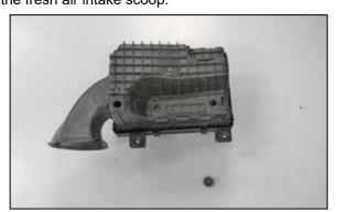
10. Remove one of the rubber mounting grommets from the factory air box.
