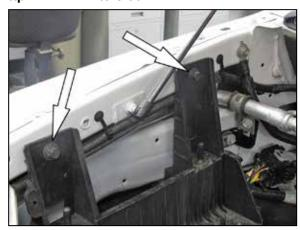
14. Remove the two factory air box mounting bracket bolts shown.
