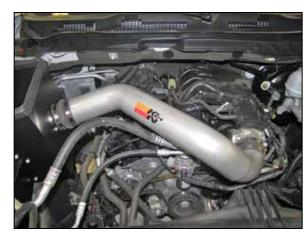
22. Install the K&N® intake tube assembly into the coupler hose at the filter adapter and then into the coupler hose at the throttle body. Adjust the tube for best fit and then secure with the provided hose clamps.
